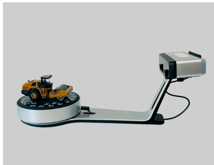
Figure 4. 3D scanner used to scan heavy construction equipment diecast models.
