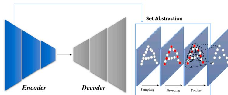
**Figure 3.** Network structure of PointNet++ (Left) and set abstraction (Right). PointNet++ obtained multi-level features by set abstraction on the encoder process, and then transmits the local–global feature into several fully connected layers and finally outputs the recognition result on the decoder process.
