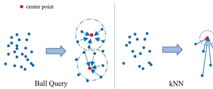
**Figure 4.** The ball query method takes the sampling point as the center of a certain radius, and selects the points within the radius ball as the neighboring points.  $k$ NN ( $K$ -nearest neighbor sampling) selects the  $K$  nearest points in coordinate space to delineate the local area.
