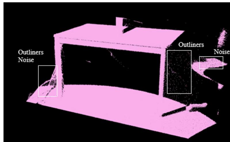
**Figure 1.** One example of the real-world point clouds with corruption (noise and outliers). Noise is a random error or bias in the point cloud acquisition process and is generally not a real value, outliers are real point cloud data that are not related to the target object.
