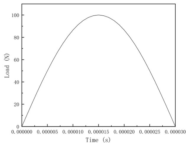
Figure 8. Half-sine periodic load.
