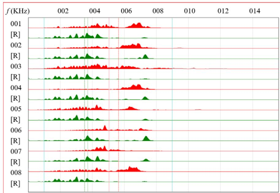
Figure 18. Tested spectrum diagram of pipeline 1 signal.
