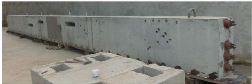
**Figure 1.** Overall view of pre-stressed bridge beam model.
