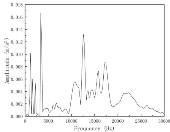
**Figure 12.** Simulated spectrum diagram of pipeline 2 signal.
