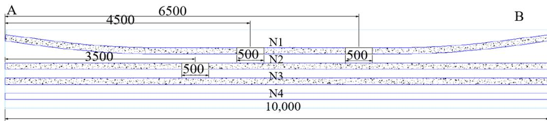
Figure 2. Model design drawing of pre-stressed beam (unit: mm).
