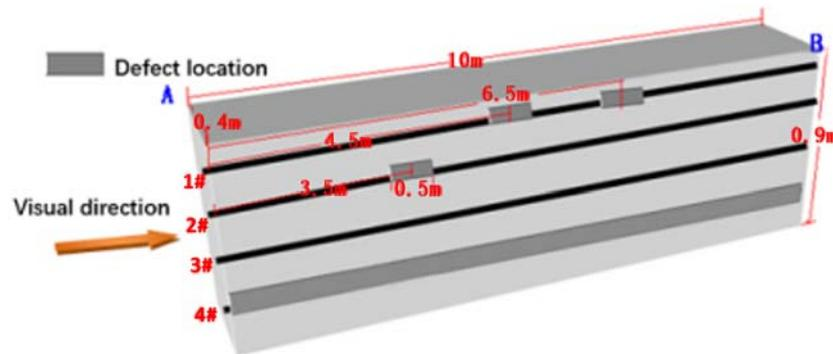
Figure 3. Model diagram of pre-stressed beam (unit: m).
