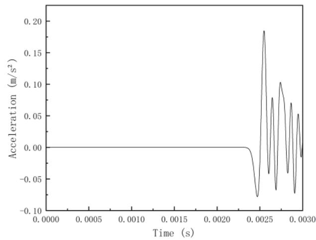
**Figure 9.** Simulated time history diagram of pipeline 1 signal.
