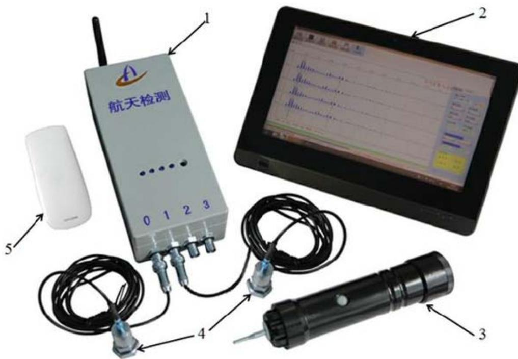
**Figure 5.** AGI-BWG pre-stressed pipeline grouting quality inspection instrument: 1—wireless data acquisition instrument; 2—iPad; 3—signal transmitter; 4—acceleration transducer; 5—wireless router.
