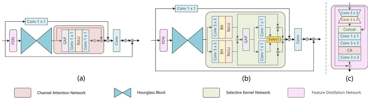
**Figure 3.** Architectures of the Attention Guiding Block (AGB): (a) is the Attention Guiding Block—Top (AGB-T); (b) is the Attention Guiding Block—Bottleneck (AGB-B); (c) is the Feature Distillation Network (FDN). Here,  $\odot$  denotes the sigmoid function.
