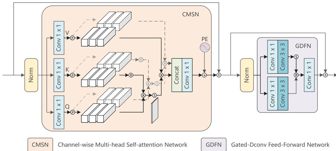
**Figure 4.** Architectures of the Channel-wise Multi-head Transformer Block (CMTB). Here,  $\textcircled{S}$ ,  $\textcircled{R}$ , and  $\textcircled{P}$  denotes the sigmoid function, reshape, and split, respectively. PE denotes the position embedding generator.
