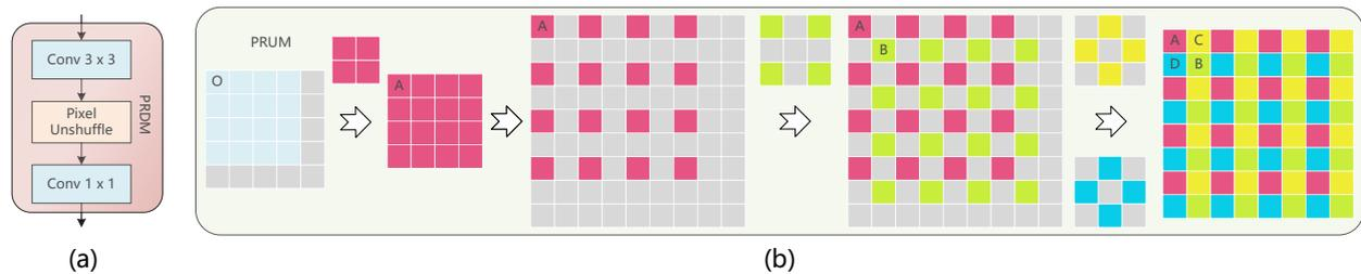
**Figure 5.** Architectures of the Pixel-Related Up/Downsample Module (PRUM/PRDM). (a) and (b) are the Pixel-Related Downsample Module and Pixel-Related Upsample Module, respectively.
