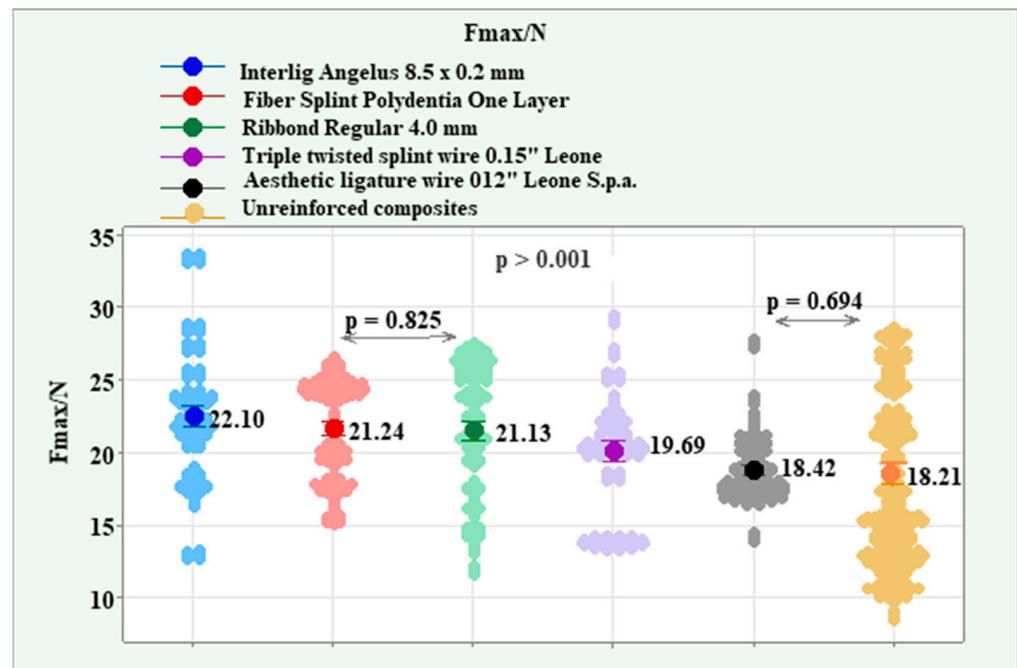
**Figure 4.** Effect of reinforcement types on maximum strength before fracture ( $F_{max}/N$ ).
