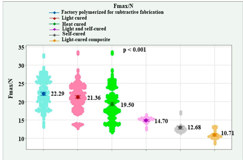
Figure 7. Effect of polymer types on maximum strength before fracture (Fmax/N).
