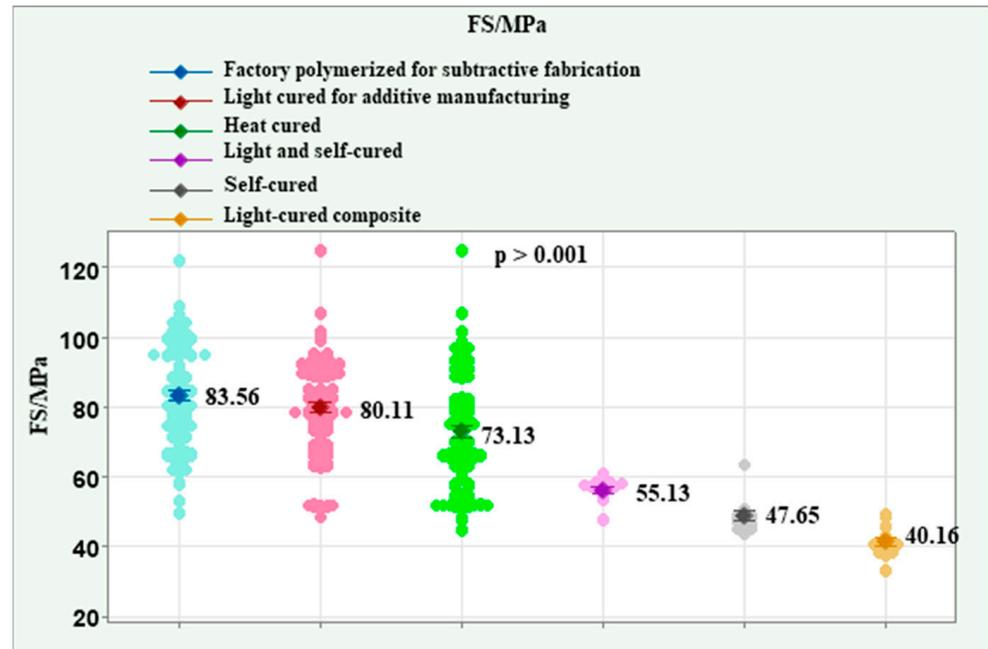
Figure 6. Effect of polymer types on flexural strength (FS/MPa).
