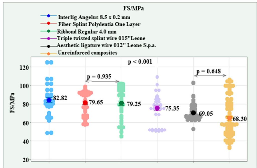
**Figure 3.** Effect of reinforcement types on flexural strength (FS/MPa).
