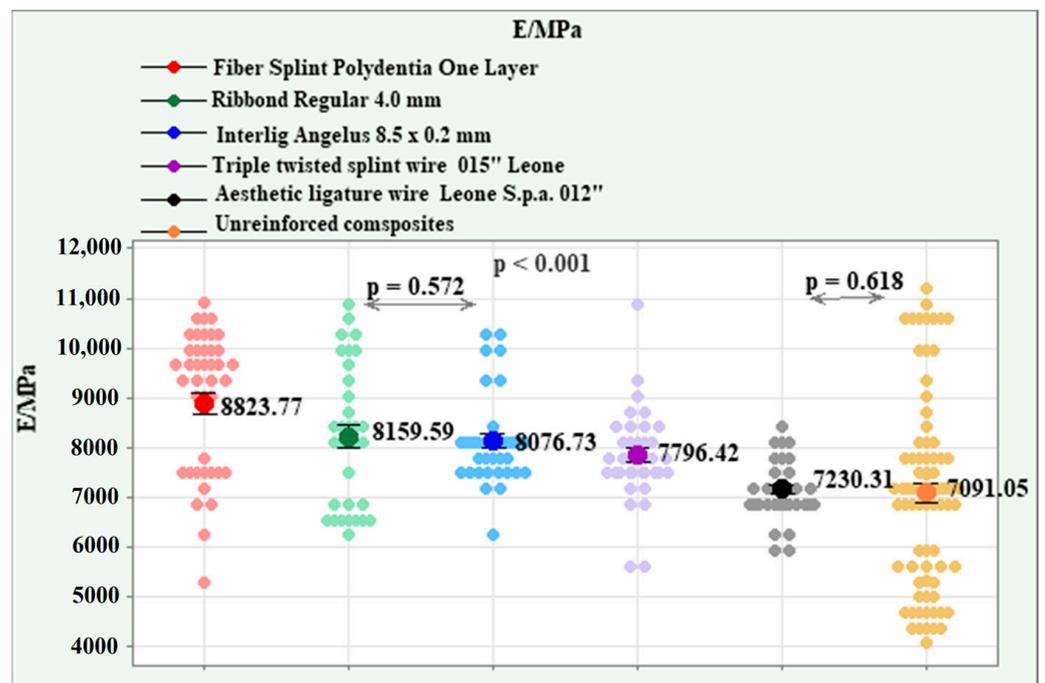
**Figure 5.** Effect of reinforcement types on modulus of elasticity (E/MPa).
