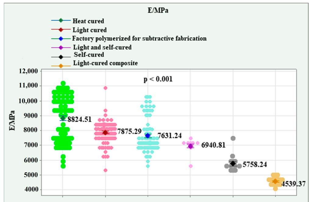
Figure 8. Effect of polymer types on modulus of elasticity (E/MPa).
