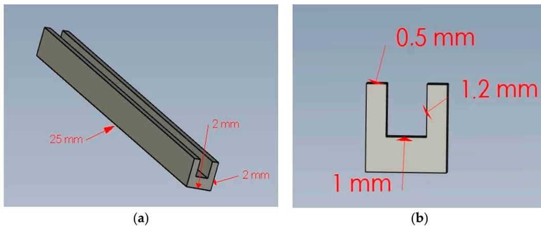
**Figure 2.** (a) A test specimen with a channel for manufacturing using CAM technologies; (b) cross section of the same object.
