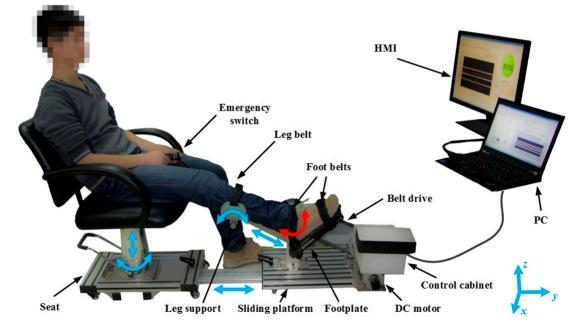
**Figure 3.** Robot-assisted therapy for lower limbs [60]. It comprises of a sliding platform, an adjustable seat, a robotic footplate, a leg support, an actuator, a control cabinet, emergency switches, and a human–machine interface (HMI). The red arrow shows the active movement of the ankle joint, while the blue arrows indicate the passive adjustable degrees of freedom. Image reused under the Creative Commons attribution license.
