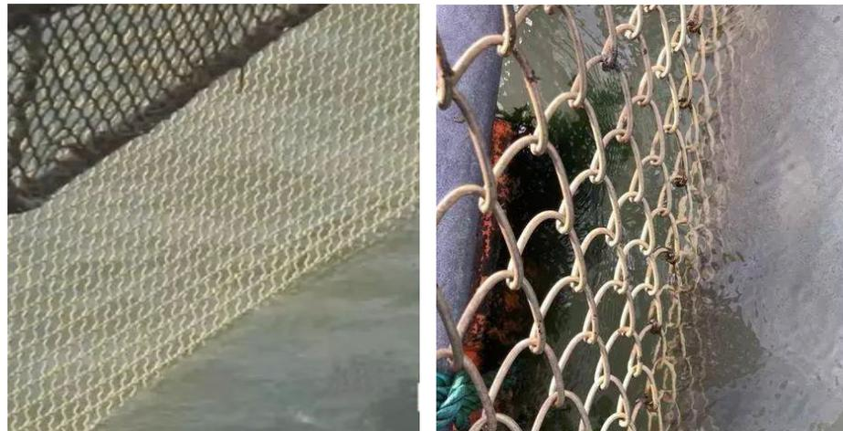
**Figure 22.** Photos of a copper alloy net used in pile–net enclosure facility.
