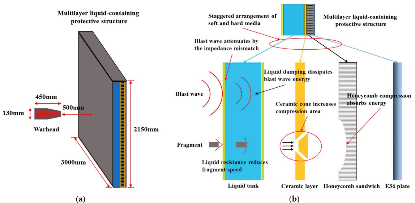
**Figure 1.** (a) A conceptual figure of the experiment performed by Huang [25]. (b) Theoretical analysis of the protection mechanism.
