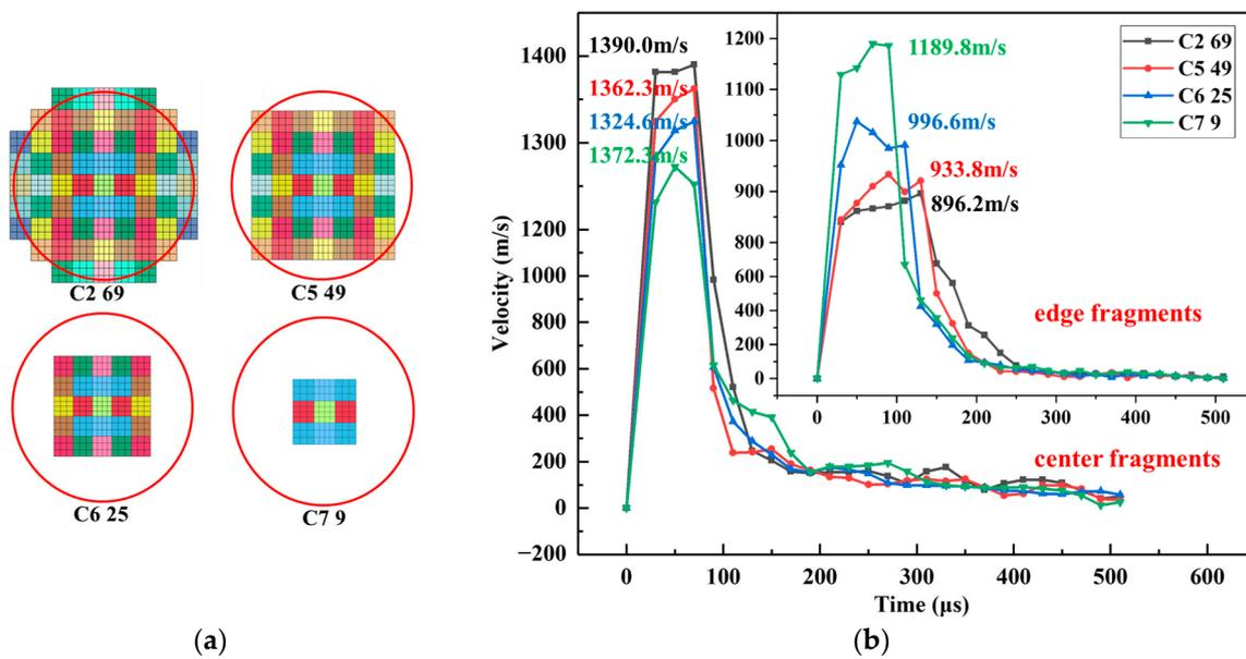
**Figure 15.** (a) Distribution of fragments with different numbers (Different colored squares are fragment groups). (b) Fragment velocity time history curve of different fragment numbers.
