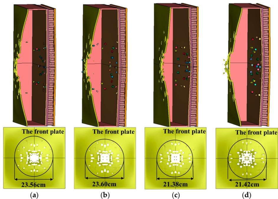
Figure 13. Ultimate response of multilayer liquid-containing protective structure and damage results of the front plate under different fragment weights: (a) C1— $6 \times 6 \times 2$  mm; (b) C2— $6 \times 6 \times 3$  mm; (c) C3— $6 \times 6 \times 4$  mm; and (d) C4— $6 \times 6 \times 6$  mm.
