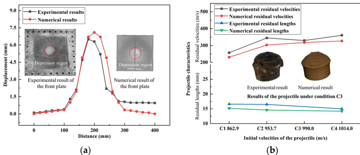
**Figure 4.** (a) Comparison of the experimental and numerical results of the front plate [37]. (b) Comparison of the experimental and numerical results of the projectile [38].
