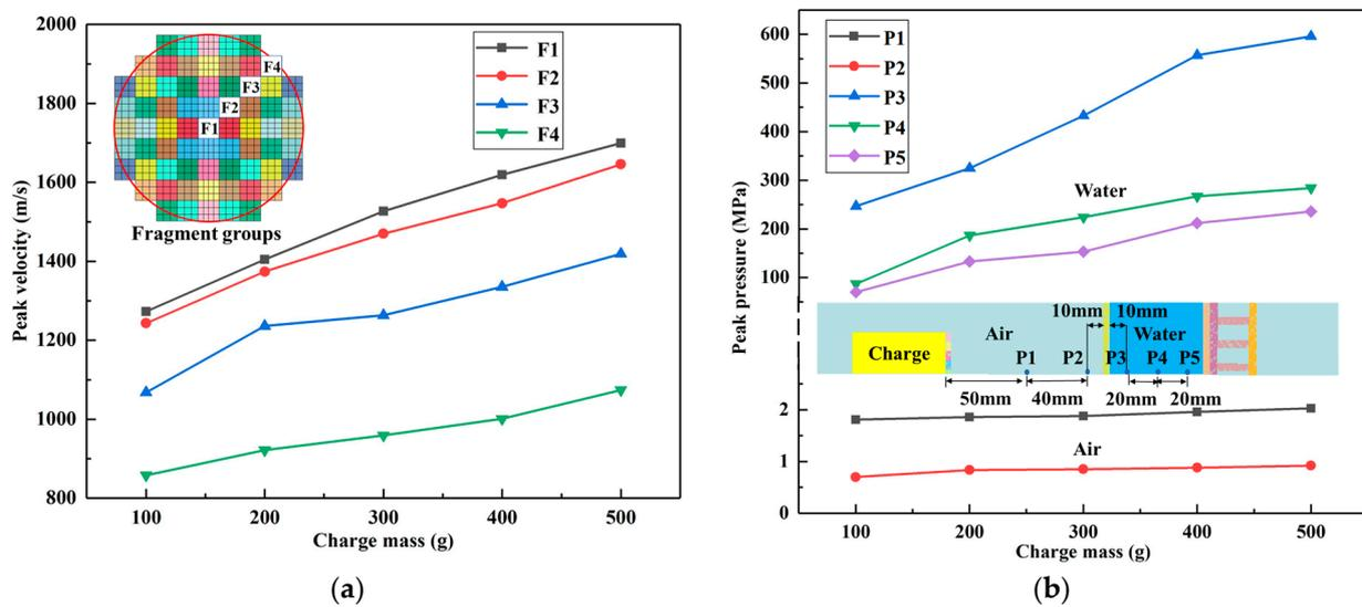
**Figure 9.** Data of measuring points under different charge masses. (a) Peak velocities of fragments at different positions (Different colored squares are fragment groups). (b) Peak pressure of different measuring points.
