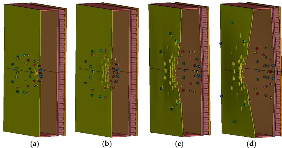
**Figure 6.** Response process of multilayer liquid-containing protective structure under combined loading (Different colored squares are fragment groups). (a) 100  $\mu\text{s}$ ; (b) 150  $\mu\text{s}$ ; (c) 300  $\mu\text{s}$ ; (d) 600  $\mu\text{s}$ .
