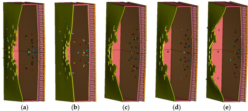
**Figure 10.** Ultimate response of the protective structure under different charge masses. (a) 100 g; (b) 200 g; (c) 300 g; (d) 400 g; (e) 500 g.
