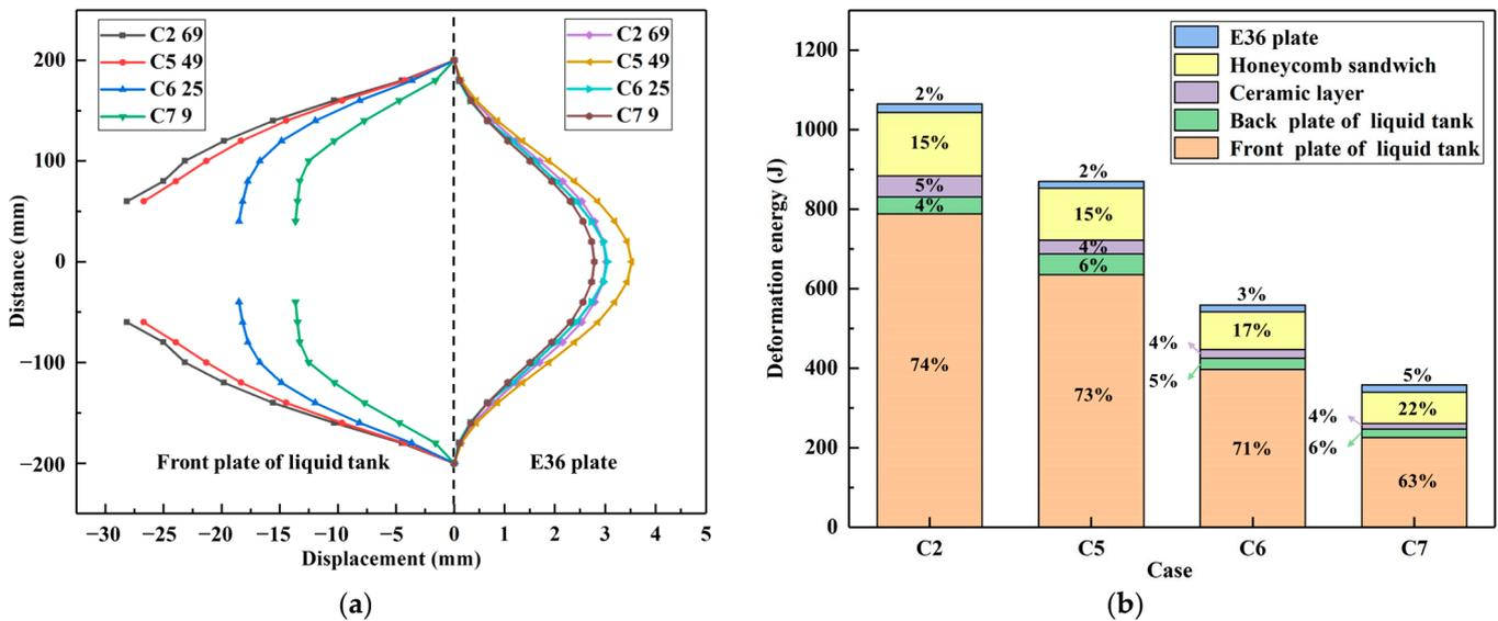
**Figure 17.** Structural response results under different fragment numbers. (a) Final deformation of foremost and rearmost plates. (b) Energy of deformation absorption and its proportion of each layer structure.
