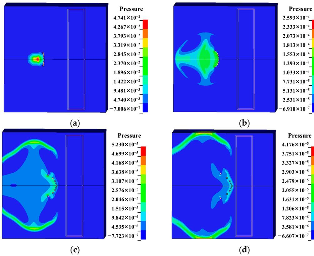
Figure 7. Evolution in air pressure (unit: 100 GPa). (a) 10  $\mu$ s; (b) 30  $\mu$ s; (c) 60  $\mu$ s; and (d) 80  $\mu$ s.
