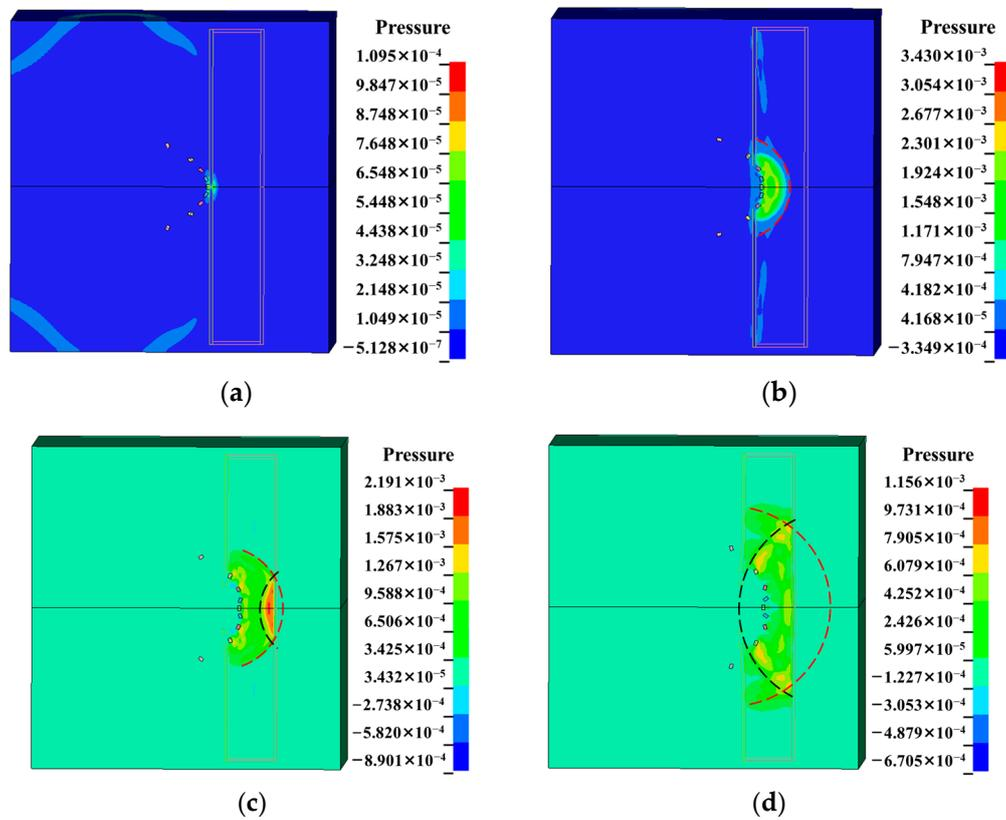
Figure 8. Evolution of water pressure (unit: 100 GPa). (a) 90  $\mu$ s; (b) 110  $\mu$ s; (c) 130  $\mu$ s; and (d) 160  $\mu$ s.
