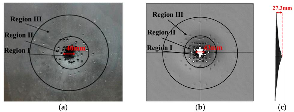
**Figure 3.** Comparison of the experimental and numerical results of the steel plate under combined loading. (a) Experimental results [36]. (b) Simulation results. (c) Numerical maximum deflection of the steel plate.
