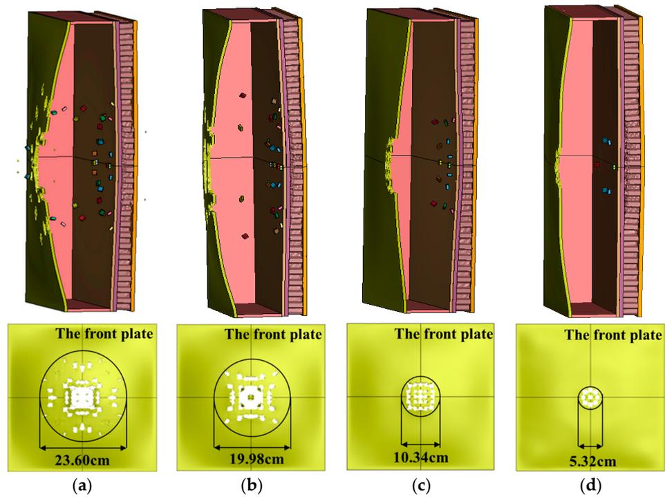
**Figure 16.** Ultimate response of multilayer liquid-containing protective structure and the damage results of the front plate under different fragment numbers. (a) C2—69; (b) C5—49; (c) C6—25; and (d) C7—9.
