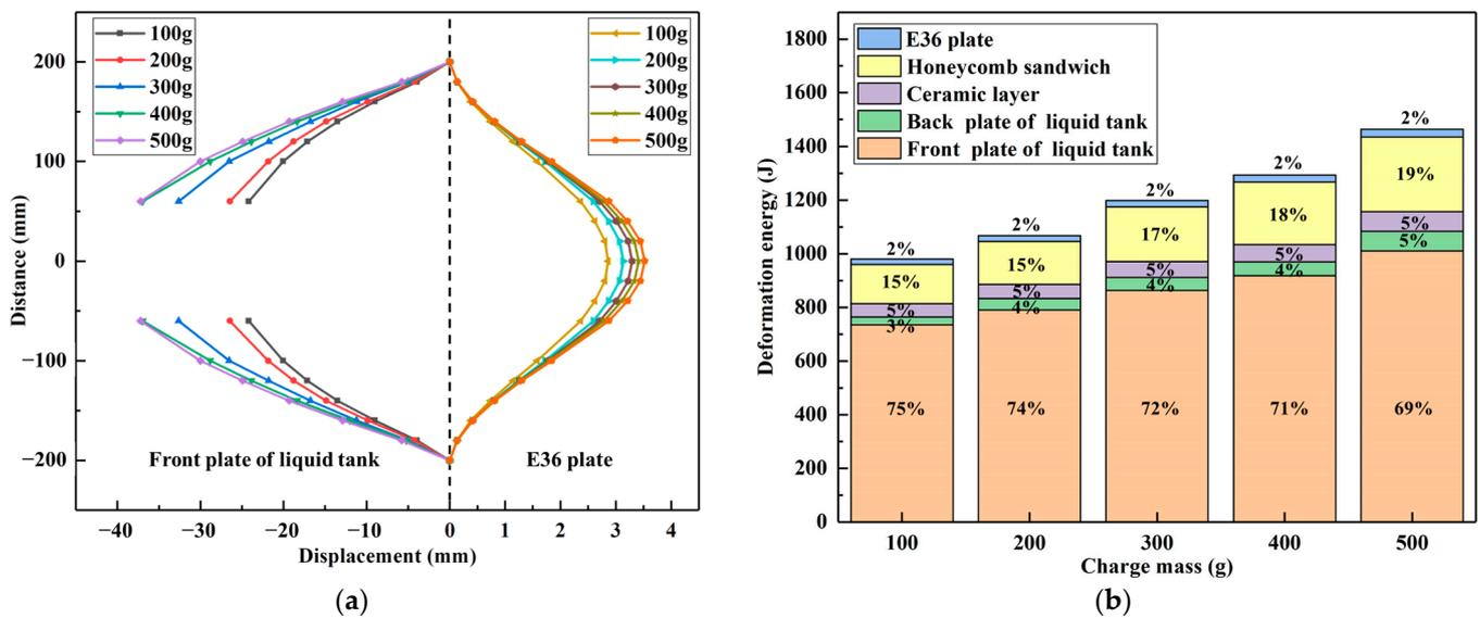
**Figure 11.** Structural response results under different charge masses. (a) Final deformation of foremost and rearmost plates. (b) Energy of deformation absorption and its proportion for each layer structure.
