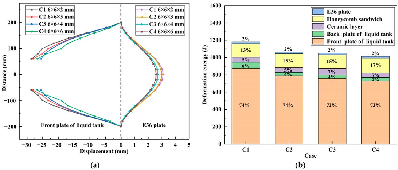
Figure 14. Structural response results under different fragment weights. (a) Final deformation of foremost and rearmost plates. (b) Energy of deformation absorption and its proportion of each layer structure.
