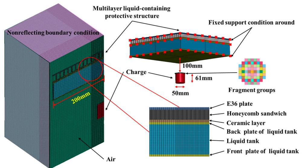
**Figure 2.** Numerical simulation model [25] (Different colored squares are fragment groups).
