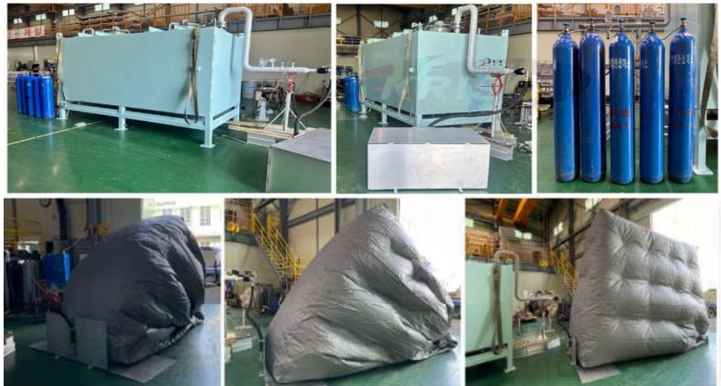
**Figure 17.** BSS prototype test for installation in a K-GTB machinery room.
