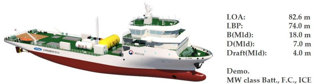
Figure 15. BSS to be equipped; 2600 GT class K-GTB appearance and specifications.
