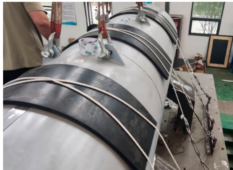
Figure 5. Tie rope ballast arrangement.
