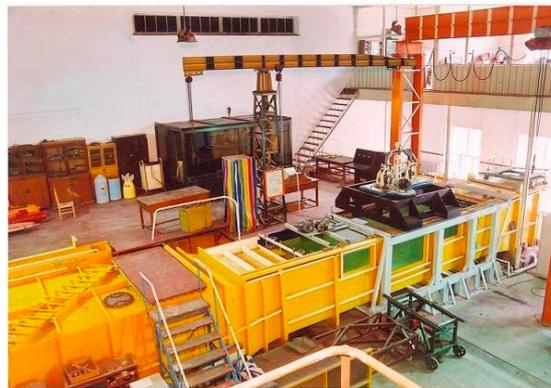
**Figure 2.** Circulating water channel for hydrodynamic test.
