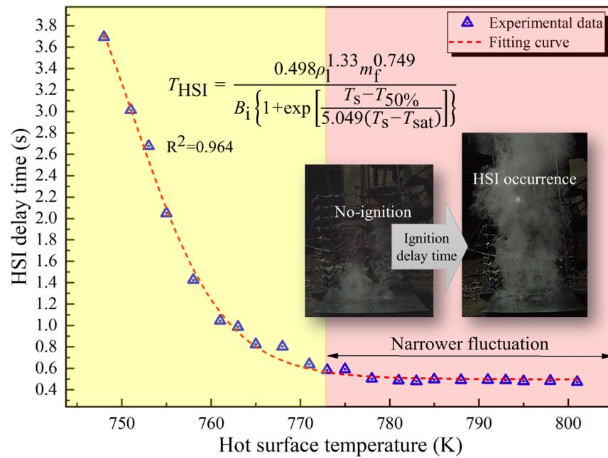
Figure 7. HSI delay time of marine diesel with changing heated surface temperatures.
