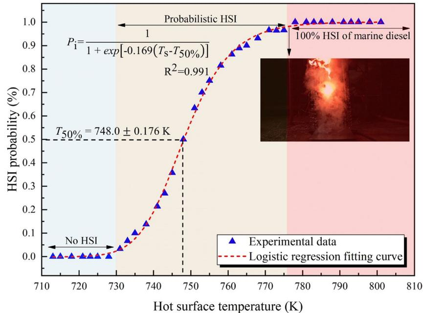
Figure 8. Trend of HSI probability with surface temperature for leaked marine diesel.
