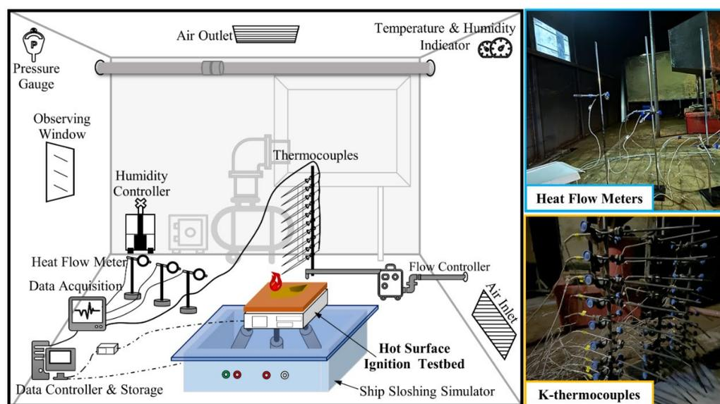
**Figure 1.** Configuration of experimental apparatus and system utilized in HSI tests.
