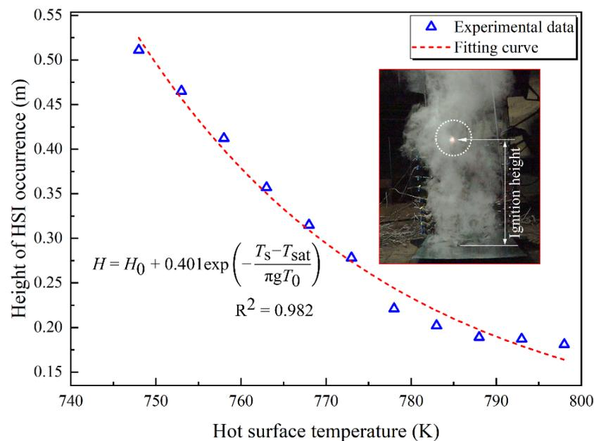
**Figure 3.** Heights at which marine diesel ignites with various heated surface temperatures.
