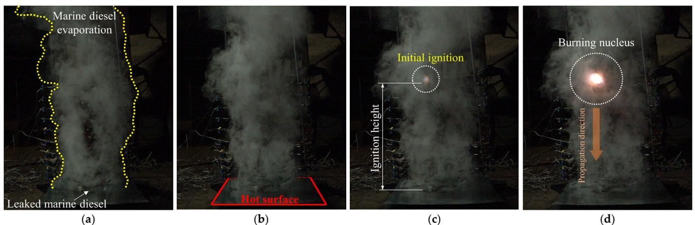
**Figure 2.** The initial ignition of marine diesel leaking onto the hot surface of a ship engine system. (a)  $t = 3.108$  s; (b)  $t = 3.675$  s; (c)  $t = 3.725$  s; (d)  $t = 3.733$  s.
