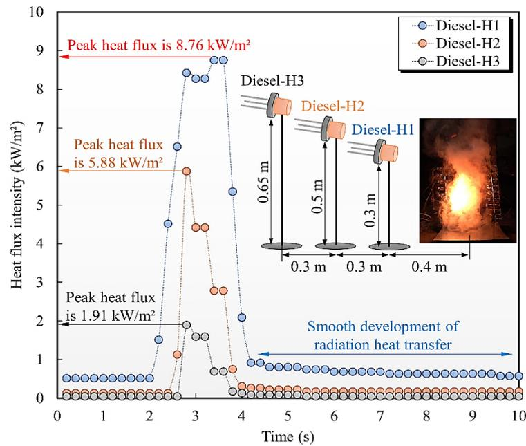
**Figure 6.** Heat flux intensities of marine diesel HSI changes with distance from the hot surface.
