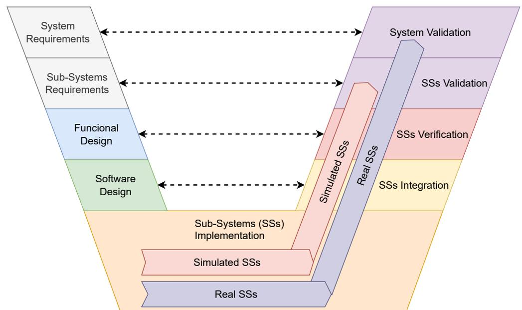
**Figure 2.** Research project development stages hybrid V-diagram. Real subsystems must be verified and validated versus simulated subsystems.
