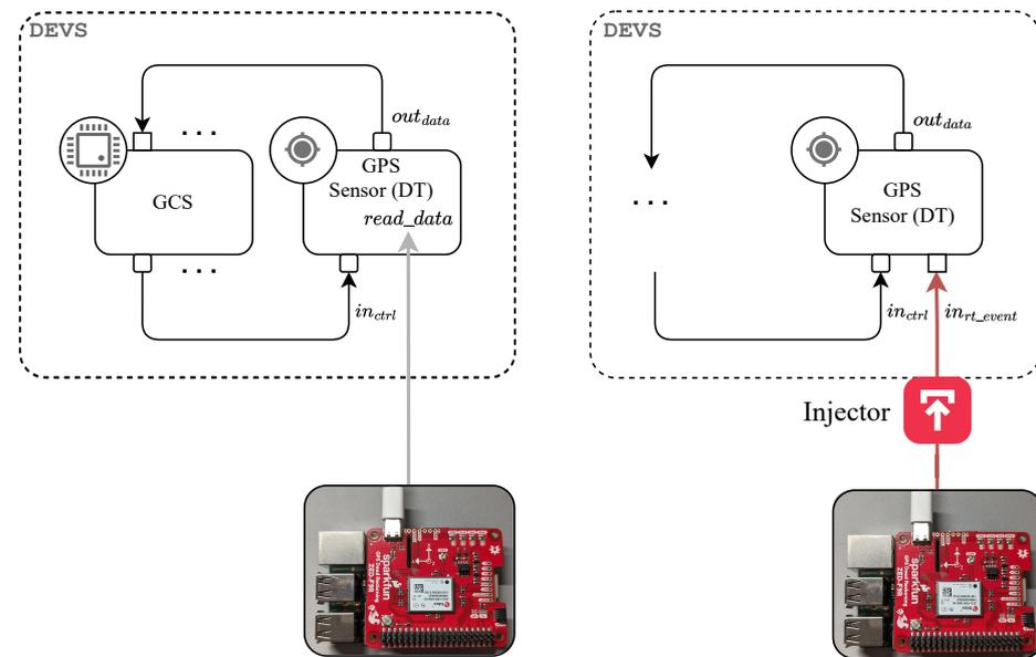
**Figure 10.** Integration of Things by polling (left) and integration of Things by event injection (right) in the simulator.
