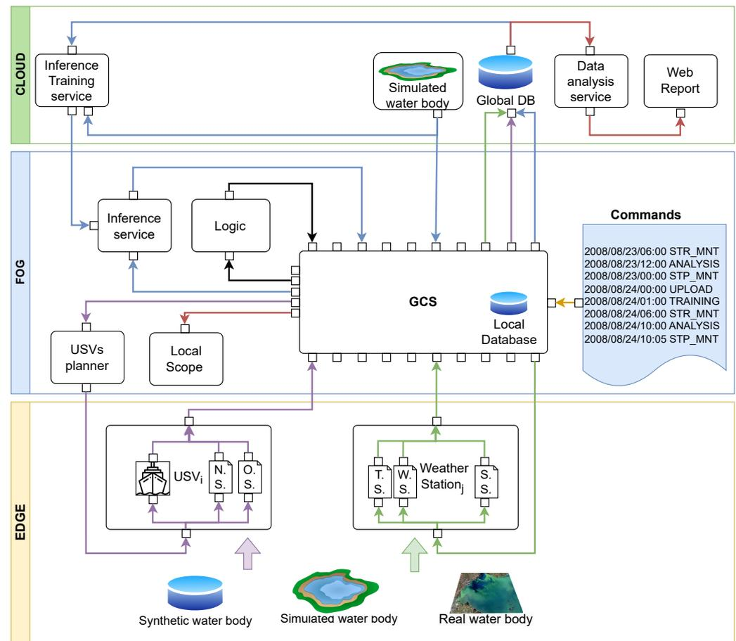
**Figure 7.** Coupled model of the architecture for bloom monitoring using an inference service.
