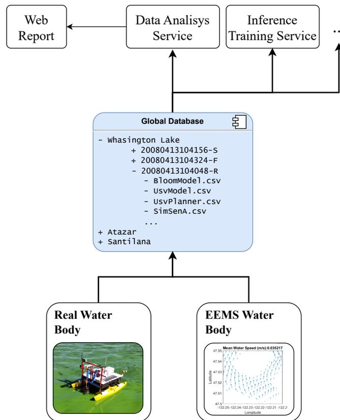
**Figure 12.** Connection structure of cloud layer with the simulator through the database.
