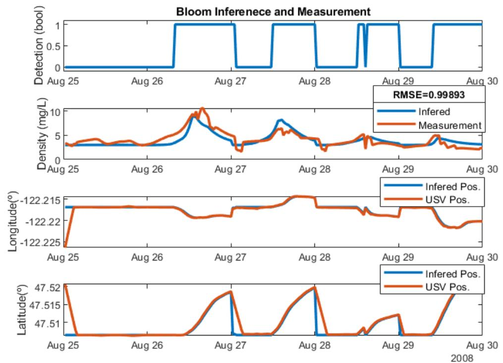
**Figure 9.** Functional verification of the inference model over several days. In the first plot, the model predicts the existence of a possible bloom. The second plot shows the density inferred by the model, the density measured by the USV, and the mean square error. The third and fourth plots show the longitudes and latitudes inferred by the bloom model and those attained by the USV.
