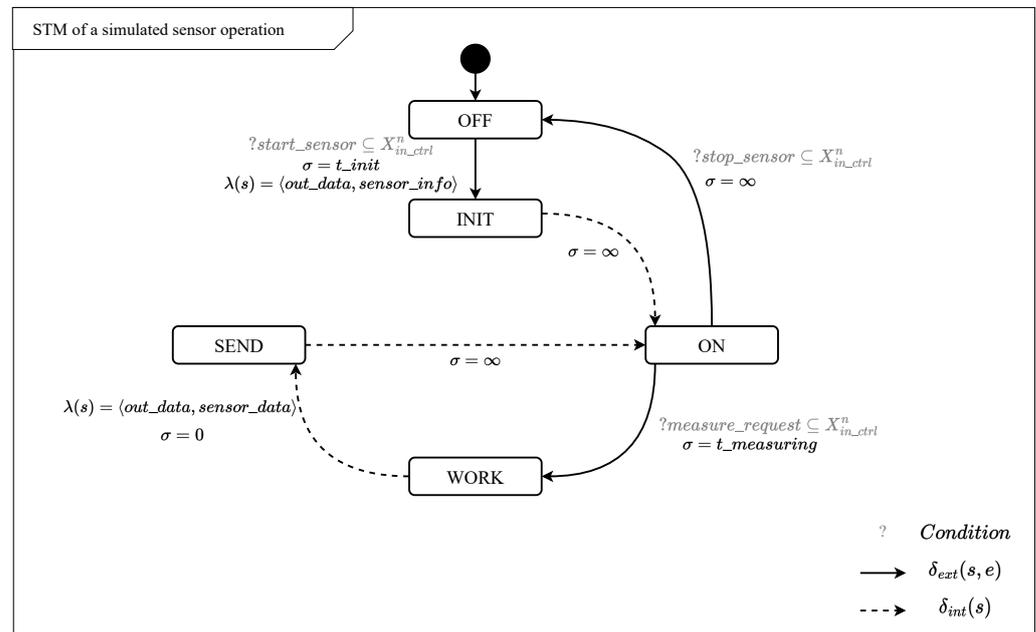
Figure 6. STM of a simulated sensor operation.
