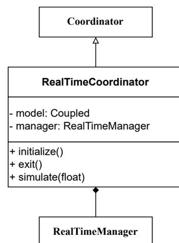
**Figure 3.** Unified Modeling Language (UML) diagram of the `RealTimeCoordinator` class.
