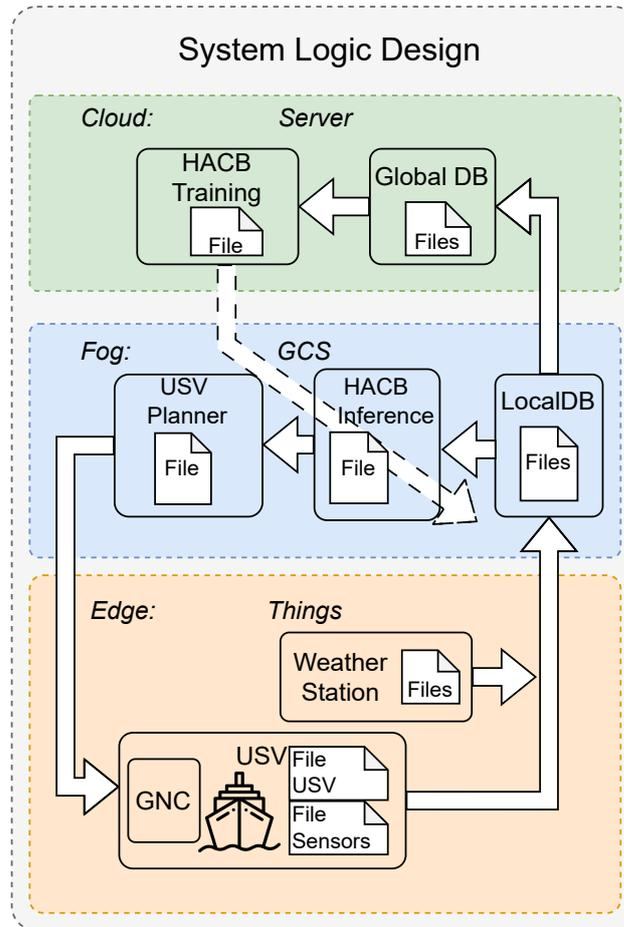
**Figure 5.** Distributed system model and information flows. Things in the edge layer capture information from the environment and feed it to the GCS, which resides in the fog layer. In this layer, the HACBs positions are inferred and the USV trajectory is planned. In parallel, all the information is uploaded to the cloud layer server to retrain the inference models. Subsequently, in a supervised way, the inference models are updated on the fog layer.
