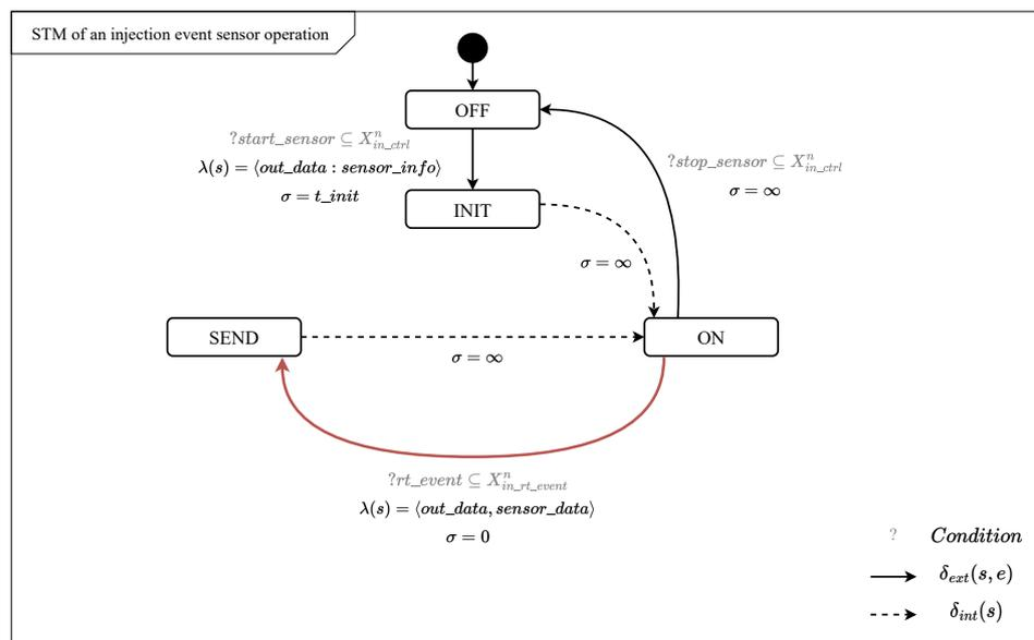
**Figure 11.** SysML state machine diagram of injection event sensor operation. The diagram forms part of a use case of the state machine diagram shown for the case of a sensor. Unlike this one, sensors implemented by event injection do not have a WORK state since their performance depends only on external events.
