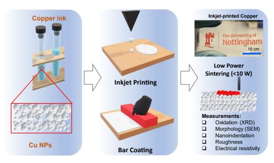
**Figure 1.** An overview of the investigation carried out in this study. Cu micro parts were developed through inkjet printing and bar coating via the direct deposition of Cu NP inks followed by low-power photonic sintering. Afterwards, various properties of the developed Cu microparts were investigated.
