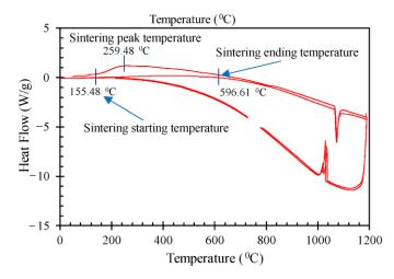
Figure 2. DSC results for Cu NP, weight corrected heat flow plotted against temperature.
