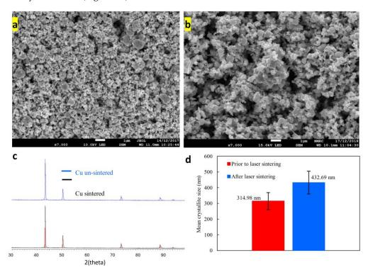
**Figure 3.** SEM images of un-sintered (**a**) and laser processed (**b**) Cu NP. The scale bar is 1  $\mu$ m. (**c**) XRD patterns of sintered and un-sintered Cu. (**d**) Mean Cu NP crystallite size before and after laser sintering.
