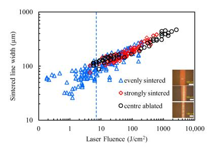
Figure 8. Sintered line width against laser fluence for a single layer of Cu NP.
