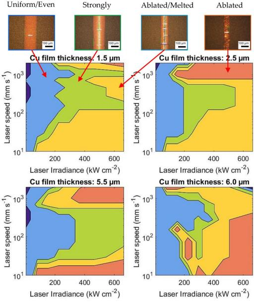
Figure 7. Process window contour maps of different sintering phenomena at varying laser irradiance and laser speeds for four different Cu film thicknesses on a glass substrate. The images and labels indicate dark blue: no effect, light blue: evenly sintered, green: strongly sintered, yellow: continuously ablated and melted, red: ablated.
