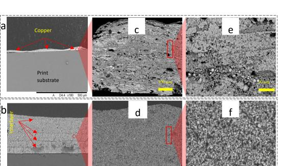
**Figure 4.** Compilation of SEM images of the cross-section of (**a**,**c**,**e**) inkjet-printed and (**b**,**d**,**f**) barcoated Cu samples.
