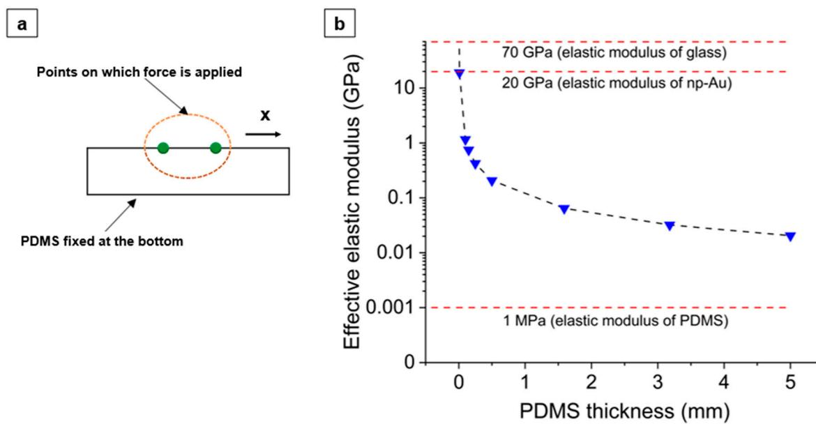
**Figure 6.** (a) Schematic showing the simulation setup to compute the effective elastic modulus of PDMS at the surface. (b) Effective elastic modulus of the PDMS substrate at the free surface as a function of the PDMS thickness. The black dashed line is a visual guide only.
