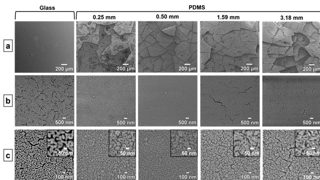
**Figure 2.** Top-view SEM images of (a) macroscopic cracks at  $150\times$ , (b) microscopic cracks at  $35,000\times$ , and (c) ligaments and pores at  $150,000\times$  magnifications in the np-Au thin films on glass and PDMS layers of varying thickness.
