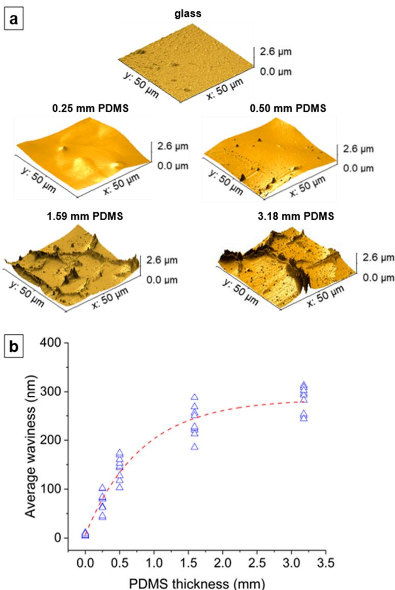
**Figure 10.** (a) AFM topographies of the np-Au film surface on glass and PDMS of different thicknesses, showing the absence of buckling in np-Au/glass and the variation in buckling in np-Au/PDMS. (b) Average waviness values of the surface topography of np-Au films as a function of PDMS thickness (zero thickness denotes the glass substrate) obtained by multiple line scans of different np-Au islands.
