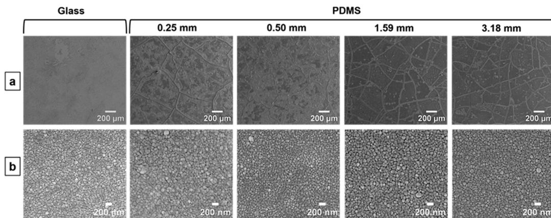
**Figure 1.** Top-view SEM images of as-deposited AuAg precursor thin films on glass and PDMS layers of varying thicknesses at (a) low ( $150\times$ ) and (b) high ( $50,000\times$ ) magnifications.
