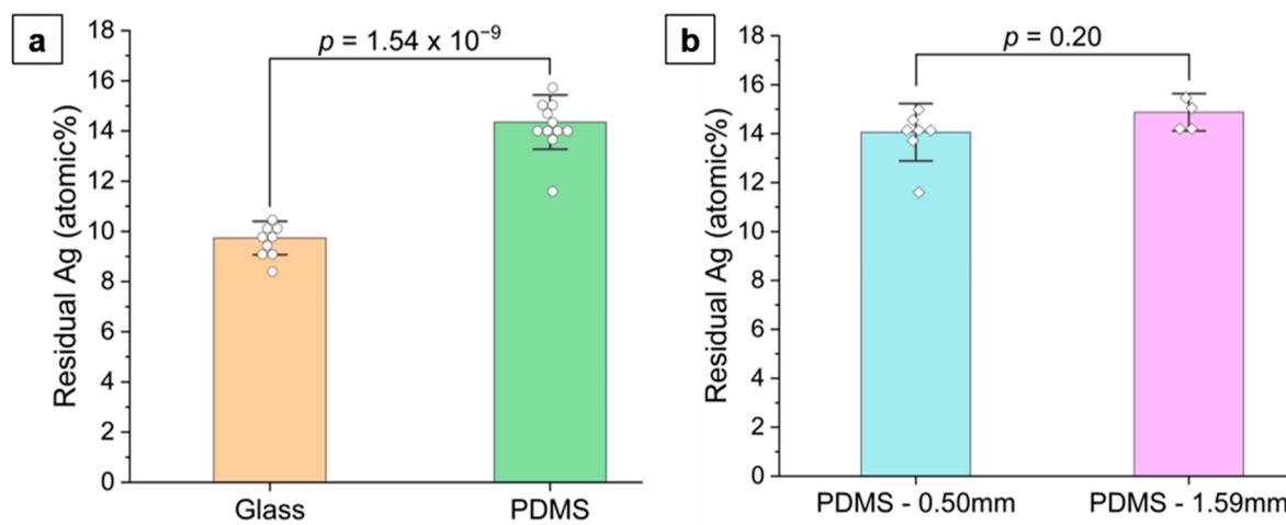
**Figure 9.** Comparison of the average residual silver content after dealloying between (a) np-Au/glass and np-Au/PDMS, and (b) np-Au/0.50 mm thick PDMS and np-Au/1.59 mm thick PDMS. A *p*-value of less than 0.05 corresponds to statistically distinct groups. The error bars show the standard deviations.
