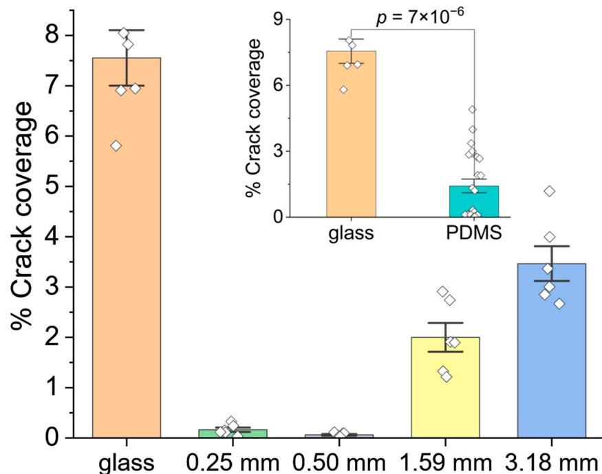
**Figure 4.** Variation in the percentage of the crack coverage in np-Au/glass and np-Au/PDMS films with varying substrate thicknesses. The inset shows the comparison of the crack coverage between np-Au/glass and the average for np-Au/PDMS films, where a  $p$ -value less than 0.05 denote a statistically significant difference. The error bars represent the standard error of the mean.
