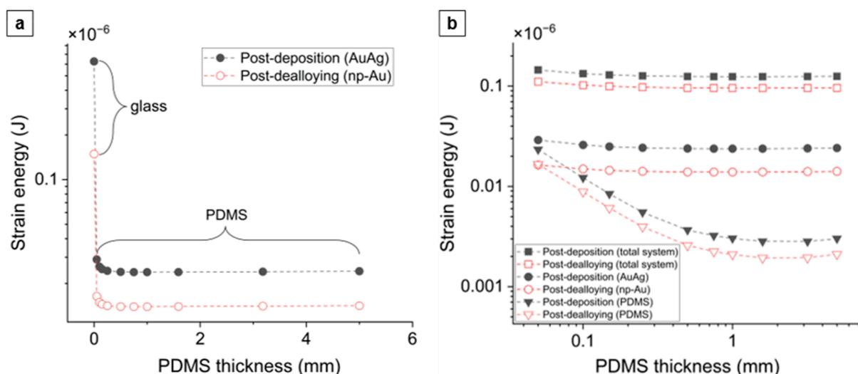
**Figure 7.** Post-deposition and post-dealloying variation in the elastic strain energy in (a) the AuAg and np-Au layers on glass and anchored PDMS of different thicknesses, and (b) the total film/substrate system, the AuAg and np-Au films, and the anchored-PDMS substrates of varying thicknesses. The y axis in (a) and both x and y axes in (b) are in log scale. The dashed lines are visual guides only.
