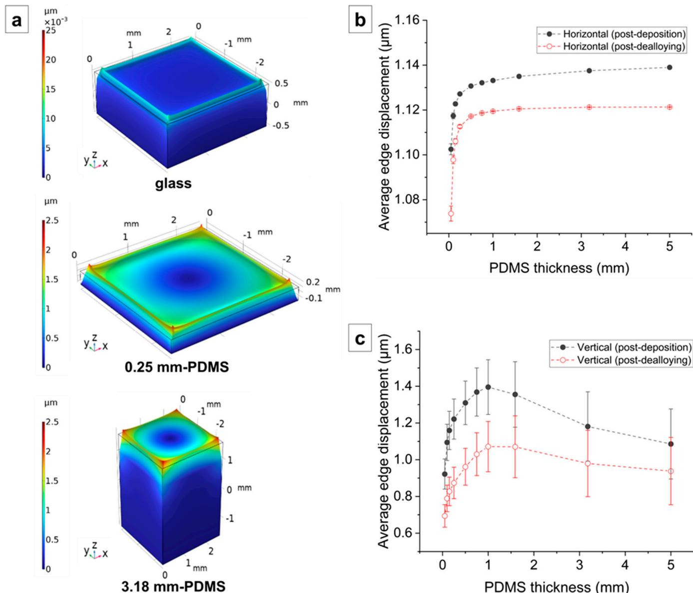
**Figure 8.** (a) Simulated deformations for post-dealloying states with representative substrate types of glass, 0.25 mm-thick PDMS and 3.18 mm-thick PDMS. Average (b) horizontal and (c) vertical post-deposition and post-dealloying edge displacements at the AuAg/PDMS and np-Au/PDMS interfaces as a function of PDMS thickness. The error bars denote standard deviation. The dashed lines are visual guides only.
