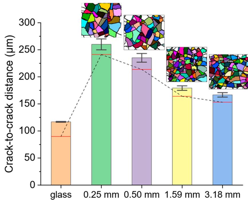
**Figure 3.** The average crack-to-crack distance for the macroscopic cracks observed in np-Au/glass and np-Au/PDMS of varying substrate thicknesses. The islands bound by the cracks in np-Au/PDMS are shown in the inset with pseudo-color segmentation for visual assistance. The red lines inside each bar denote the median crack-to-crack distance and the dashed line goes through the median values. The error bars denote the standard error of the mean.
