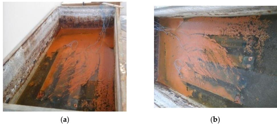
**Figure 3.** The accelerated corrosion process. (a) Three days of accelerated corrosion. (b) Eight days of accelerated corrosion.
