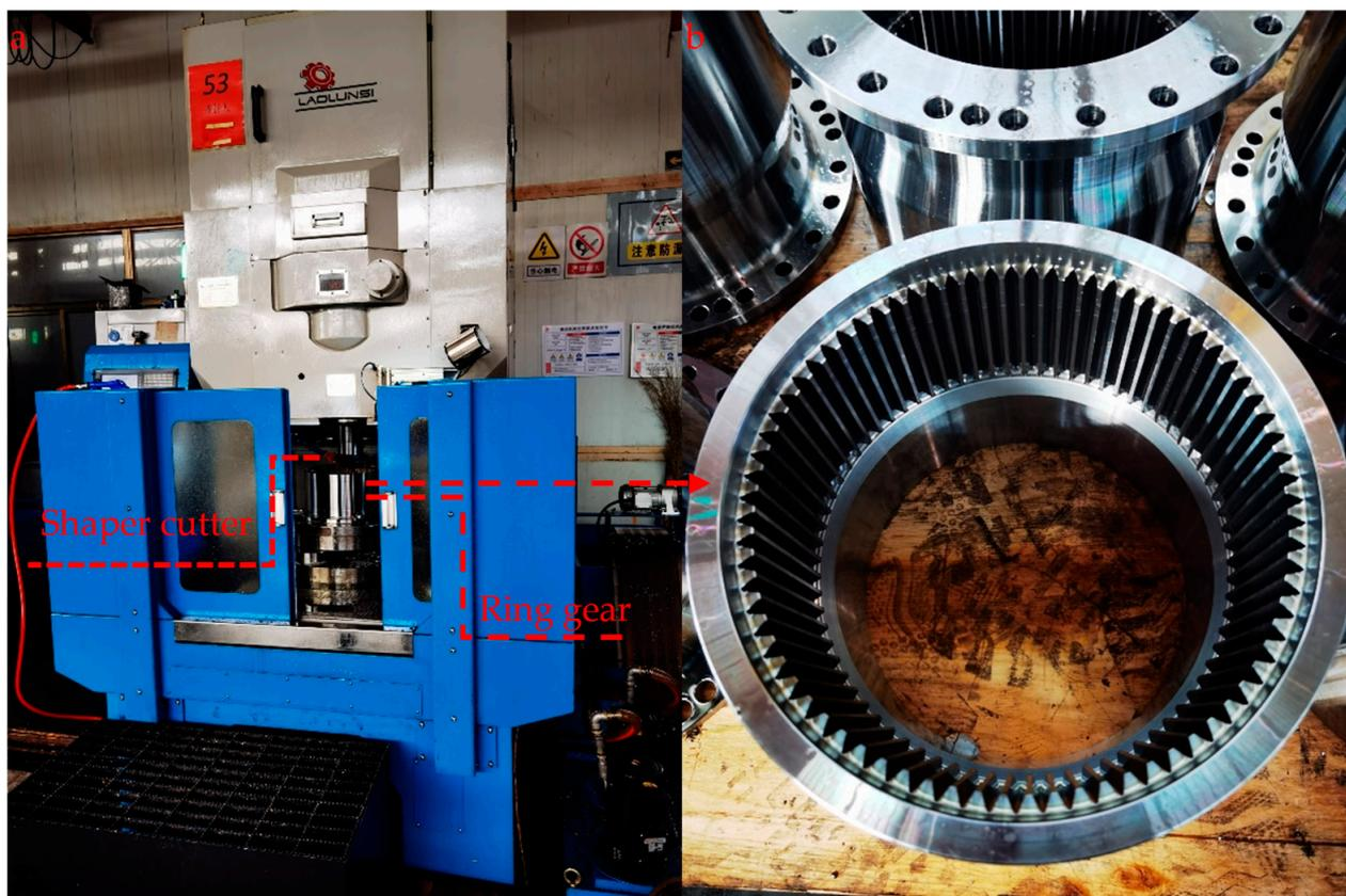
**Figure 7.** Schematic illustration of experimental setup (a) and the ring gear (b).
