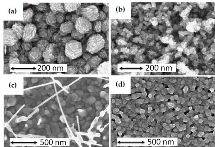
**Figure 2.** Surface morphologies of Zn films deposited on glass substrates with magnetron sputtering: (a) Ar, 2 mTorr; and (b) Ar + O<sub>2</sub>, 2 mTorr. Surface morphology of ZnO films formed by thermal oxidation of Zn films at 600 °C in air for 1 h: (c) deposited in Ar, 10 mTorr; and (d) deposited in Ar + O<sub>2</sub>, 10 mTorr. Adapted with permission from [35]; Copyright 2005 Elsevier.
