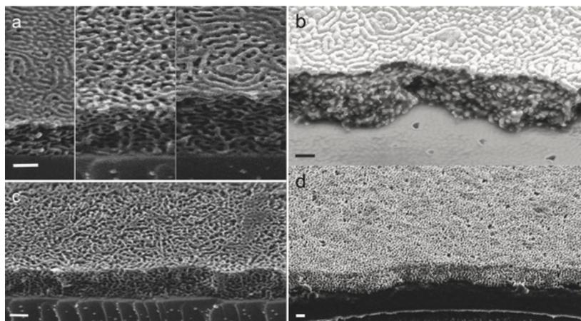
**Figure 10.** SEM of ZnO replication of the worm-like morphology: (a,c) worm-like PS template; (b) as-deposited ZnO-PS hybrid; (d) ZnO morphology after annealing at 400 °C followed by etching of the top compact layer. Scale bar are 200 nm. Reproduced with permission from [124]; Copyright 2014 John Wiley & Sons, Inc.
