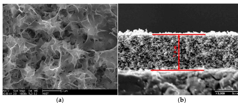
**Figure 7.** Examples of porous ZnO morphologies obtained by sol-gel methods. (a): a typical FESEM image of ZnO thin solid films deposited via a modified chemical bath deposition method. Scale bar is 2 μm. Reproduced with permission from [106]; Copyright 2006 Elsevier. (b): Cross-section FESEM image of ZnO films prepared at 0.05 mol/L methanolic zinc acetate solution and sintered at 500 °C. Scale bar is 5 μm. Reproduced with permission from [107]; Copyright 2005 Elsevier.
