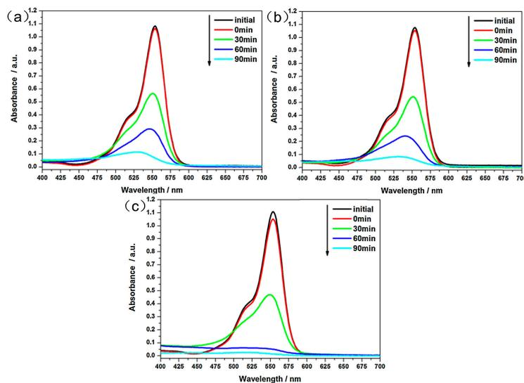
**Figure 6.** Absorbance spectra of Rhodamine- $\beta$  dye aqueous solutions under UV irradiation, in presence of ZnO nanorod arrays (ZNRAs), synthesized for different electrodeposition times: (a) one time; (b) three times; and (c) six times. Reproduced with permission from [97]; Copyright 2014 Elsevier.
