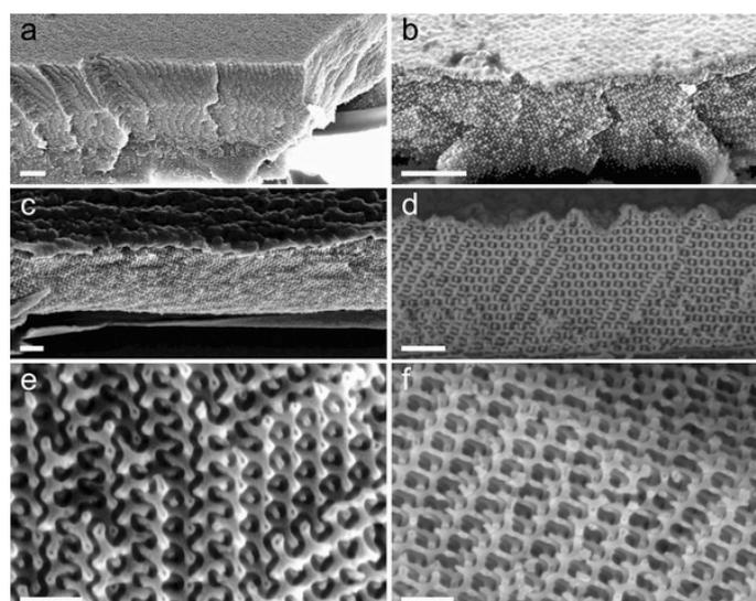
**Figure 9.** Side-view SEM images at a 45° angle of gyroid replication into ZnO: (a) gyroid PS template; (b) as-deposited ZnO-PS hybrid; (c) ZnO gyroid after annealing at 550 °C; (d–f) different faces of the ZnO gyroid shown in (c). Scale bars are 1 μm for panels (a,b), 400 nm for (c,d), 200 nm for (e,f). Reproduced with permission from [124]; Copyright 2014 John Wiley & Sons, Inc.
