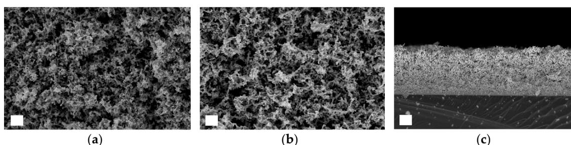
**Figure 3.** Field Emission Scanning Electron Microscope images of porous Zn thin films: (a) as-prepared; (b,c) after conversion into ZnO by thermal oxidation. Scale bar for (a) and (b) is 400 nm, for (c) is 2 μm.
