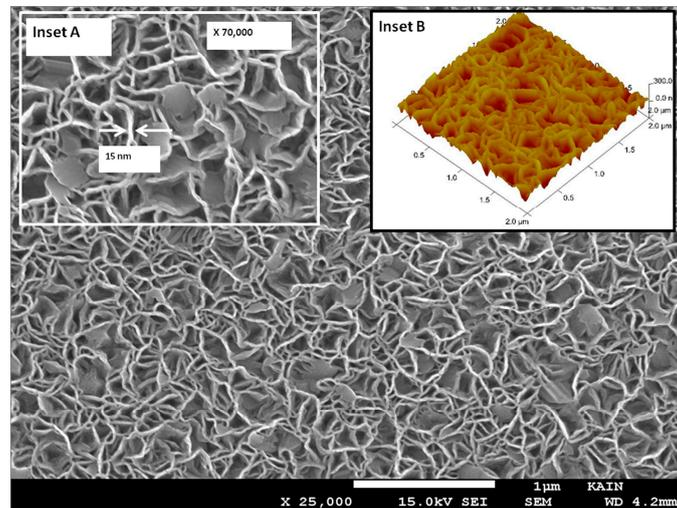
**Figure 4.** Low-magnification scanning electron microscope image and atomic force microscope profile of the 3D ZnO nanowall network grown vertically on Si(100) at 550 °C under 0.5 Torr O<sub>2</sub> background pressure. Scale bar is 1 μm. Reproduced with permission from [51]; Copyright 2015 Elsevier.
