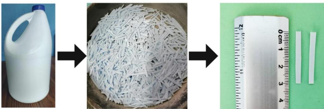
**Figure 1.** HDPE long recycled fiber.
