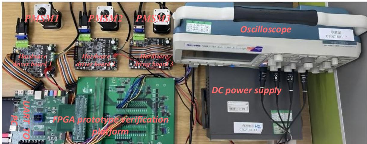
Figure 16. Diagram of the experimental platform.
