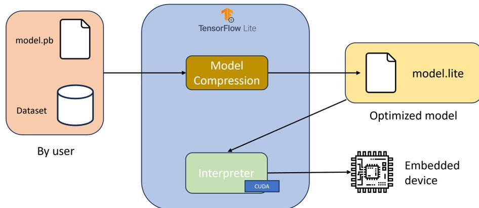
**Figure 4.** Overview of the model optimization for inference on an embedded device with NVIDIA GPU support.
