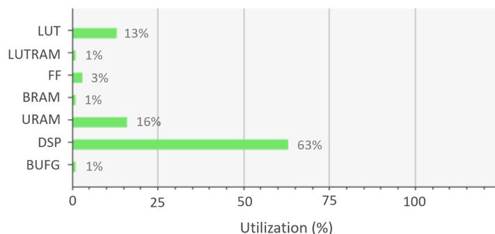
**Figure A3.** Resource usage on the Xilinx Ultrascale+ ZU7EV FPGA for the accelerator generated by FPG-AI in the highest parallelism configuration.
