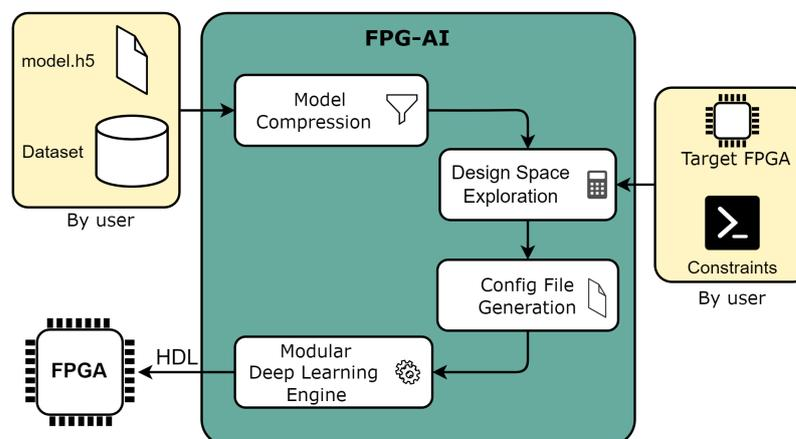
**Figure 5.** FPG-AI end-to-end tool flow.
