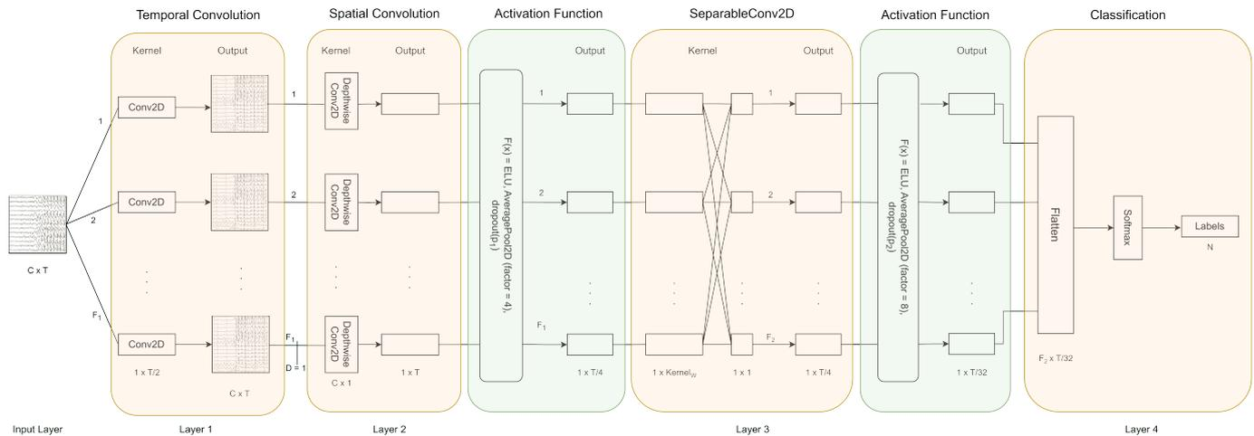
**Figure 3.** Architecture of EEGNet neural networks.
