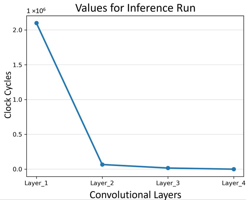
**Figure A1.** Clock cycles spent in each convolutional layer per inference run on FPGA technology.
