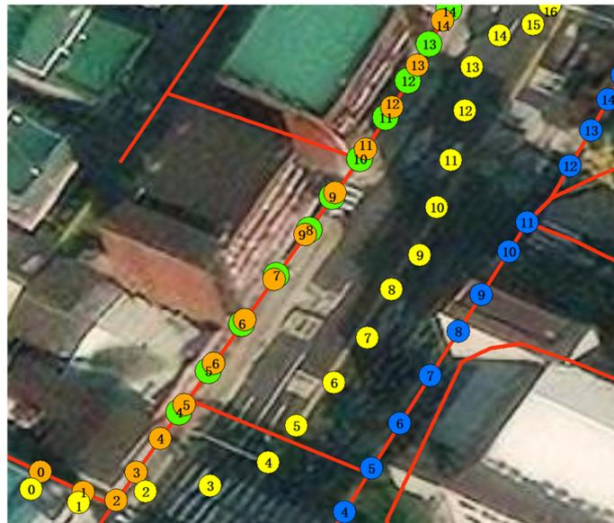
**Figure 13.** Visualization of map-matching results on the Dataset I using the probabilities of initial states based on the traditional (blue) and the proposed (green) methods.
