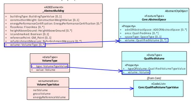
**Figure 11.** Mapping the volume attribute of \_*AbstractBuilding* in the Energy ADE for CityGML 2.0 (on the left) to the volume attribute of *AbstractSpace* in CityGML 3.0 (on the right). The corresponding complex data types are matched accordingly.
