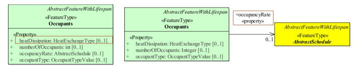
**Figure 27.** The property *occupancyRate* represented in-line and highlighted in red (left) equals the by-reference representation (right).
