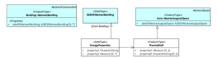
**Figure 8.** Example of extending the existing CityGML 3.0 class *AbstractBuilding* by means of the ADE hook mechanism (*EnergyProperties*, via *ADEOfAbstractBuilding*) and by deriving a new class (*ThermalHull*) from the existing class *AbstractLogicalSpace*.
