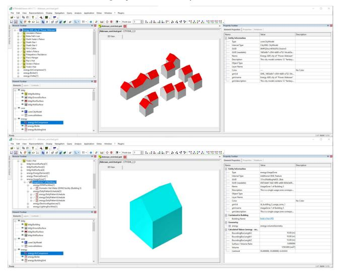
**Figure 30.** Visualisation of the test dataset in the FZK ModelViewer. Upper picture: the CityModel with its LOD2 buildings and properties. Lower picture: the *UsageZone* of Building "Yoda's Hut" with its properties and own geometry.
