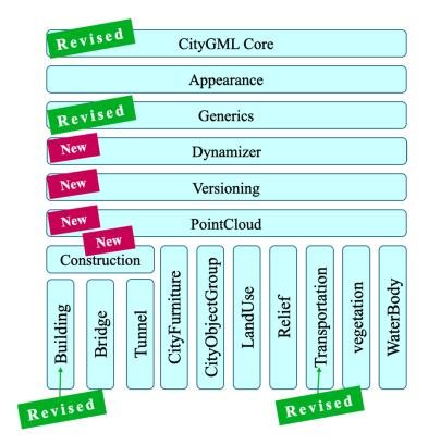
Figure 3. The modules in CityGML 3.0. Image adapted from [10].
