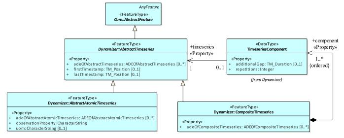
Figure 28. Excerpt of the CityGML 3.0 Dynamizer module.
