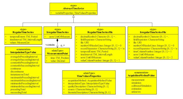
Figure 22. The time series classes in the Energy ADE for CityGML 2.0.
