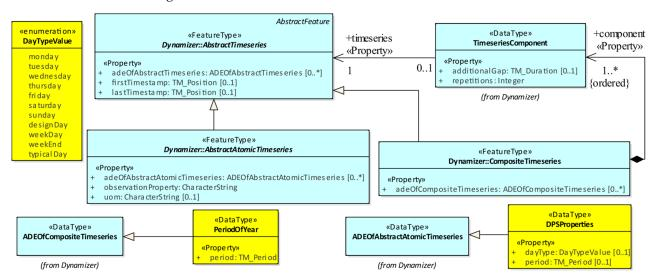
**Figure 29.** Excerpt of the CityGML 3.0 Dynamizer module (in cyan) with the added properties (in yellow) to map the DailyPatternSchedule.
