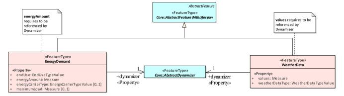
**Figure 23.** Excerpt of the Energy ADE for CityGML 3.0, showcasing the UML modelling of time-varying properties.
