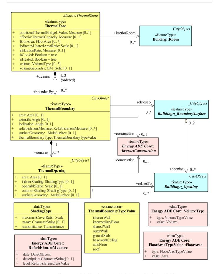
Figure 12. The Building physics module in the Energy ADE for CityGML 2.0.
