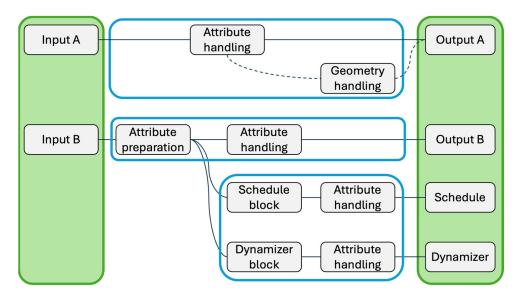
**Figure 31.** Schematic overview of the data conversion from Energy ADE for CityGML 2.0 to Energy ADE for CityGML 3.0 in FME. The "Input A" block stands for input class A, e.g., *ThermalZone*, and the "Output A" block for the respective output after the conversion. Unlike in CityGML 2.0, the *Schedule* and *Dynamizer* now have their own classes in the Energy ADE for CityGML 3.0, which is why they also have their own blocks to write the final output.
