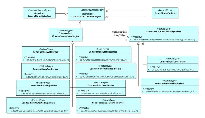
Figure 16. Excerpt of the CityGML 3.0 Construction module showing the different thematic surfaces.
