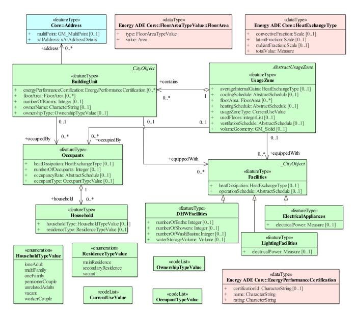
Figure 18. The Occupant behaviour module in the Energy ADE for CityGML 2.0.
