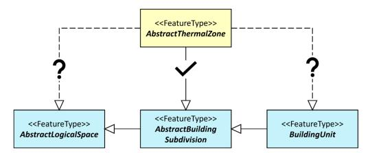
**Figure 15.** Example of several options for the parent class of *AbstractThermalZone*. Eventually, *AbstractBuildingSubdivision* is chosen.
