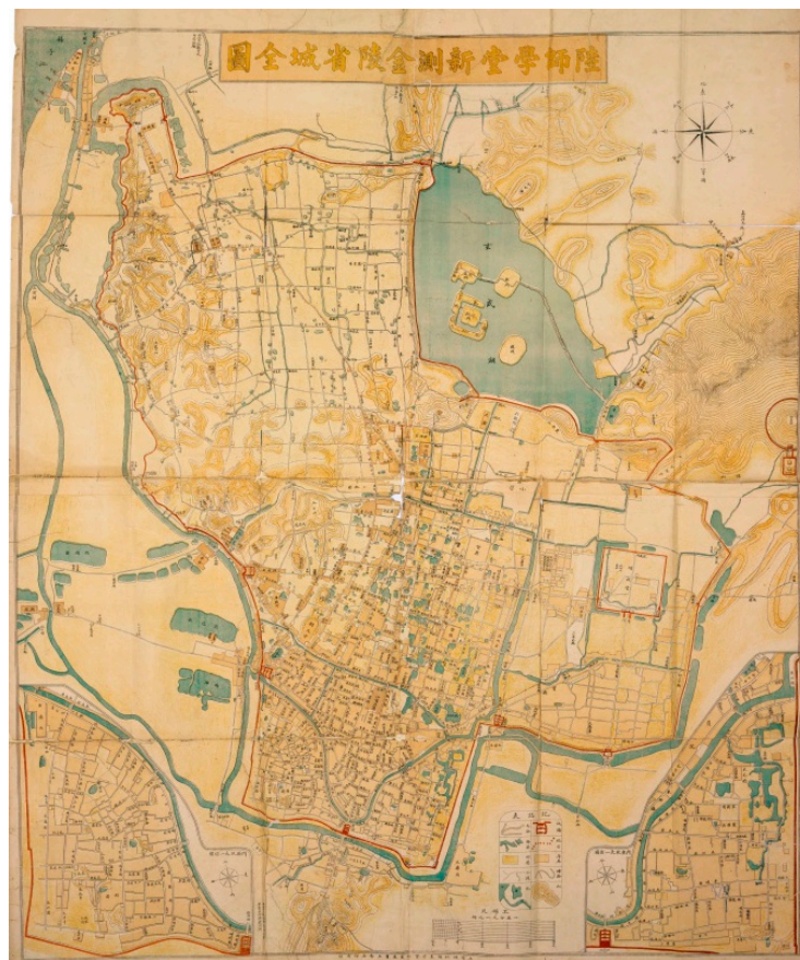
Figure A2. The New Survey Map of the Provincial City Jinling by the Army Academy (1909) [101] is the earliest map of Nanjing measured by the Chinese using modern surveying and mapping techniques. The scale of the map is 1:10,000. This map is used to define the scope of the study area.
