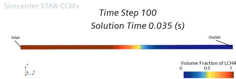
**Figure 3.** CFD model results the LCH<sub>4</sub> take 0.035 s to reach half way of the line from inlet towards the outlet. The inset scale shows the volume fraction the LCH<sub>4</sub>.
