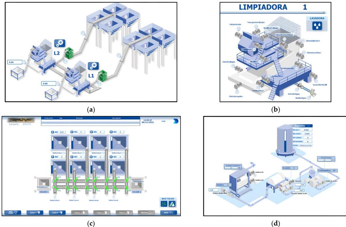
**Figure 3.** Detail of 3D SCADA screens to monitor different areas of the mill: (a) reception area; (b) cleaning area; (c) grinding area (under hoppers); (d) grinding area (grinder, mixer, decanter, and centrifuge).
