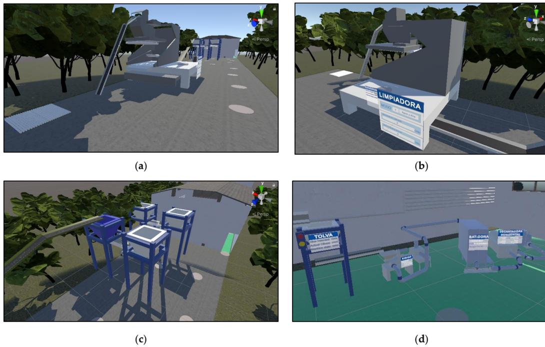
**Figure 4.** Details of the virtual environment developed for different areas of the mill: (a) reception area; (b) cleaning area; (c) grinding area (under hoppers); (d) grinding area (grinder, mixer, decanter, and centrifuge).
