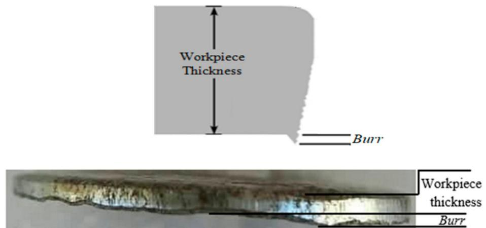
Figure 4. Blanking burr during cutting operation.
