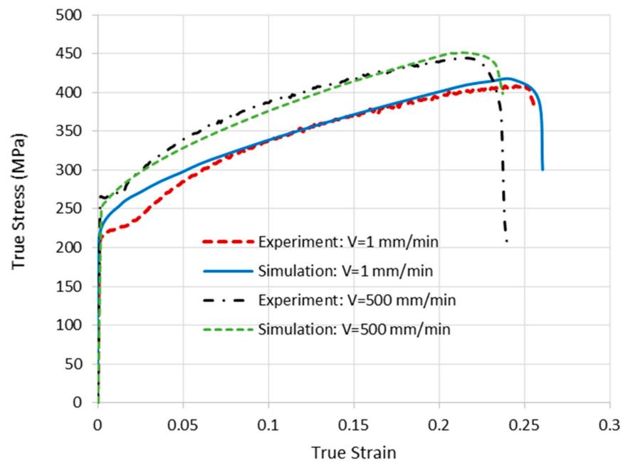
**Figure 8.** Comparison between predicted and experimental results in tensile test: true stress–strain curve.
