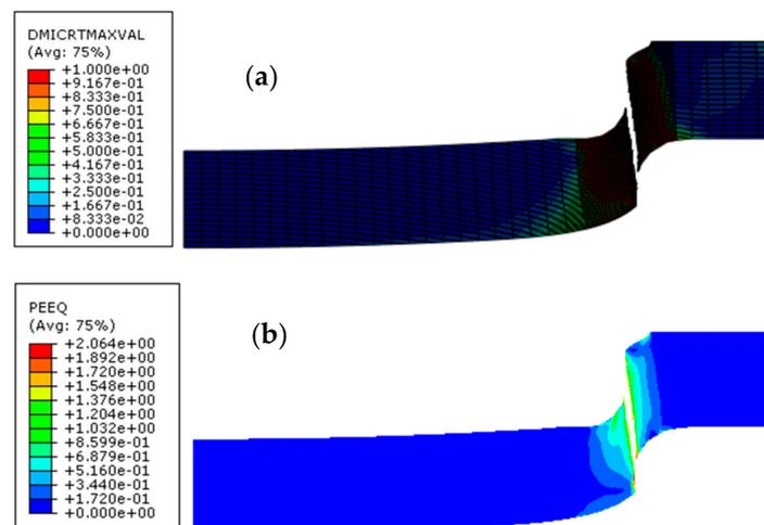
**Figure 10.** Numerical results: (a) damage fields, (b) strain fields.
