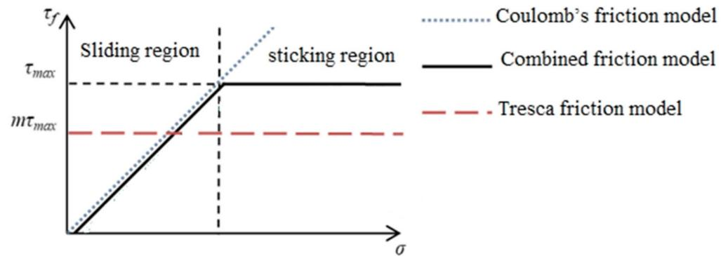
Figure 3. Friction models in blanking process.
