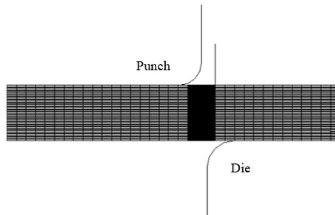
**Figure 9.** Numerical model sheet blanking operation.
