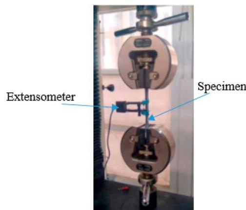
**Figure 1.** Experimental set-up of tensile test.
