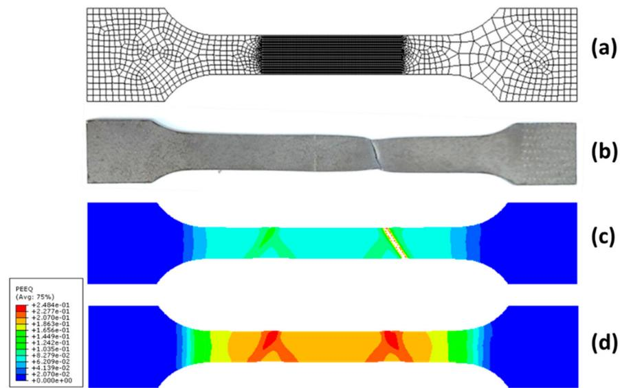
**Figure 7.** Tensile test specimens: (a) mesh size; (b) experimental test ( $V = 500$  mm/min); (c) numerical test ( $V = 500$  mm/min); (d) equivalent plastic strain distribution.
