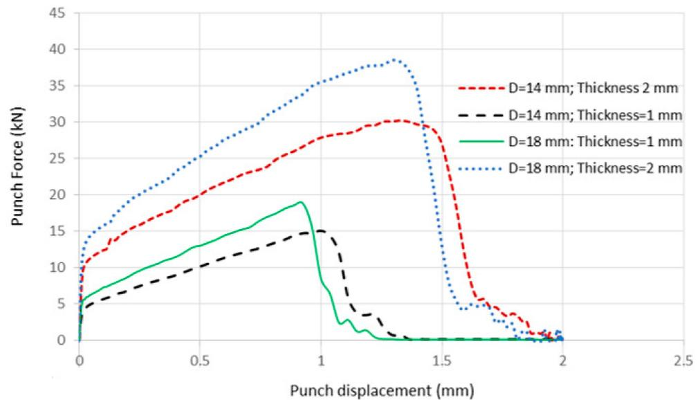
**Figure 11.** Thickness effect: punch force vs. punch displacement for  $j = 10\%$ .
