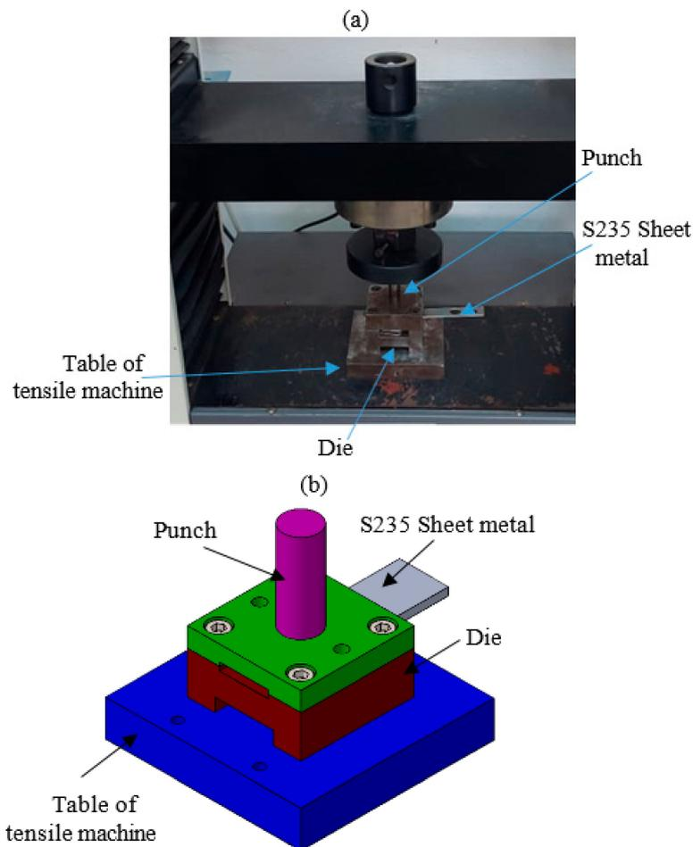
**Figure 2.** Experimental blanking tool: (a) tools and strip during blanking test; (b) 3D design of blanking tool.
