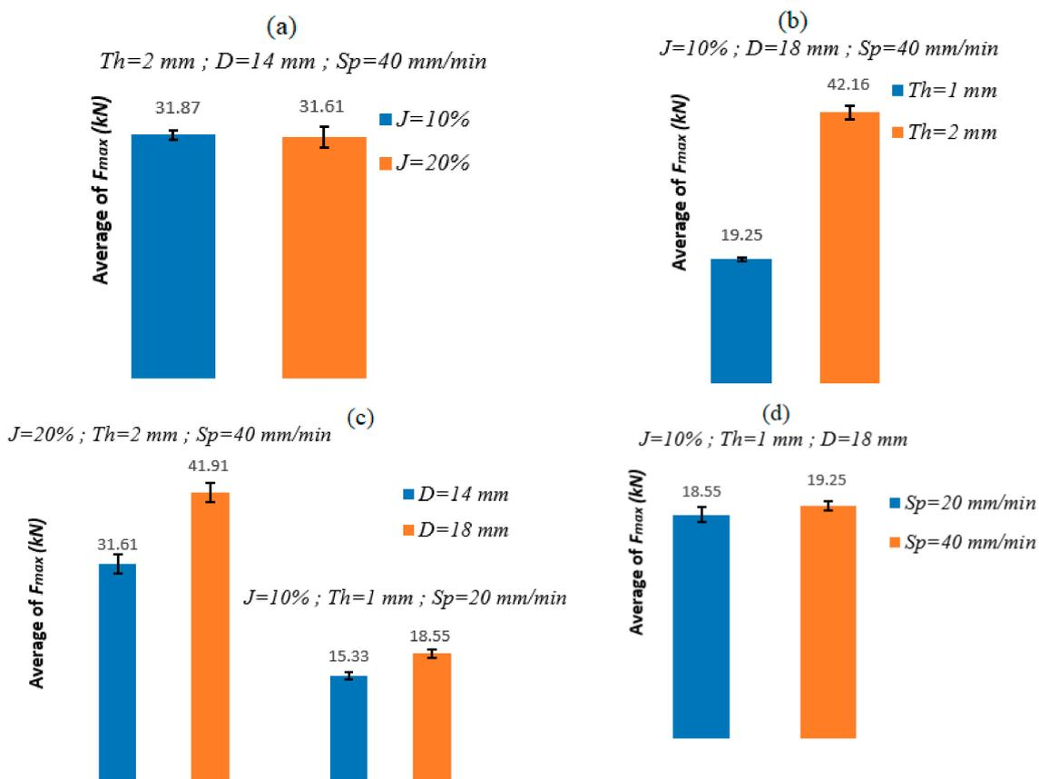
**Figure 6.** Variation of  $F_{max}$  as a function of blanking parameters.
