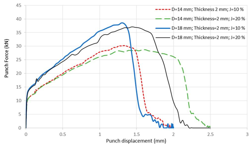
**Figure 12.** Clearance and punch diameter effects: punch force vs. punch displacement.
