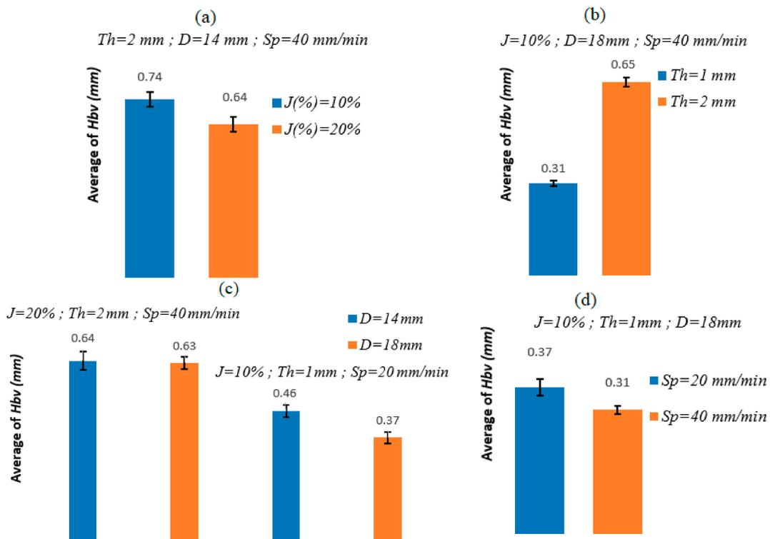
Figure 5. Variation of  $Hbv$  as a function of blanking parameters.
