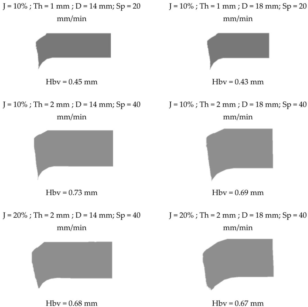
Figure 14. Predicted  $Hbv$  with different blanking parameters.
