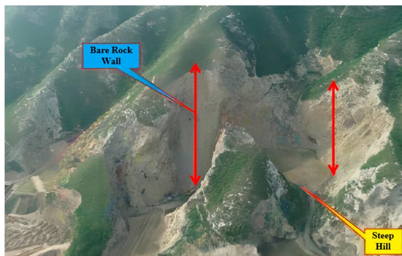
**Figure 14.** Distribution of exposed rock walls and residual hills in Zhubei Quarry #1.
