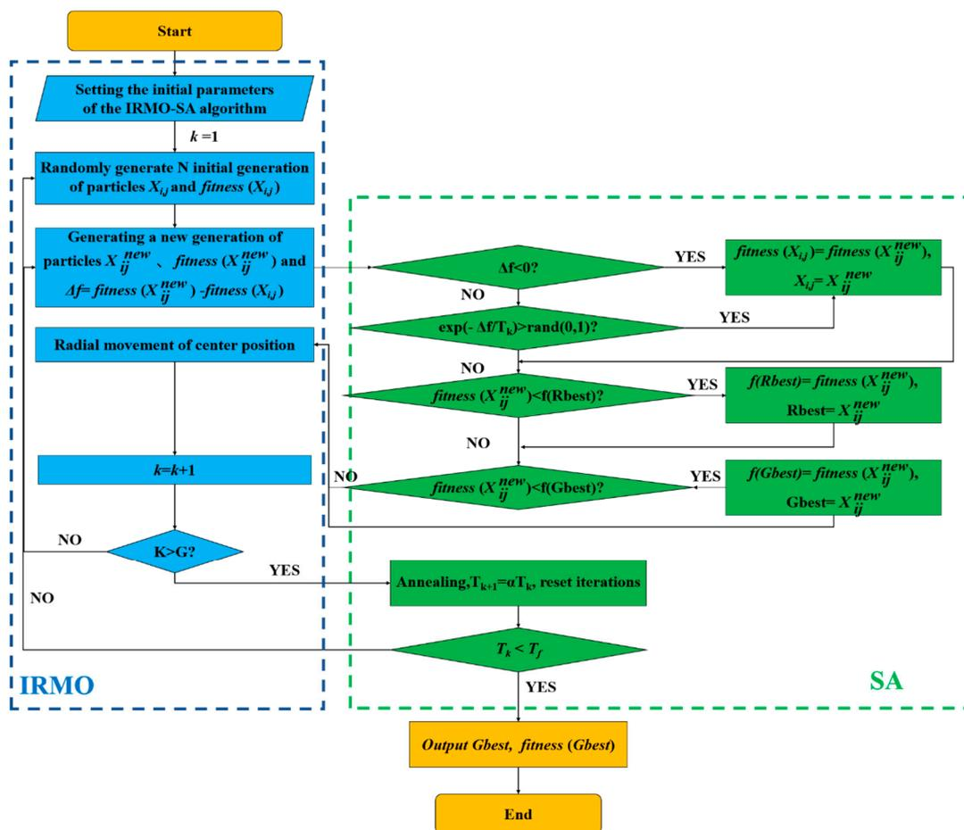
Figure 4. The flowchart of the IRMO-SA algorithm.
