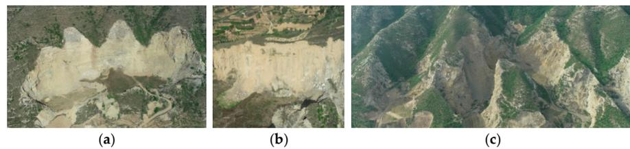
**Figure 9.** Status of abandoned open-pit mine slopes in Yellow River Basin: (a) Yanhua Quarry; (b) Torch Quarry; (c) Zhubei Quarry #1.
