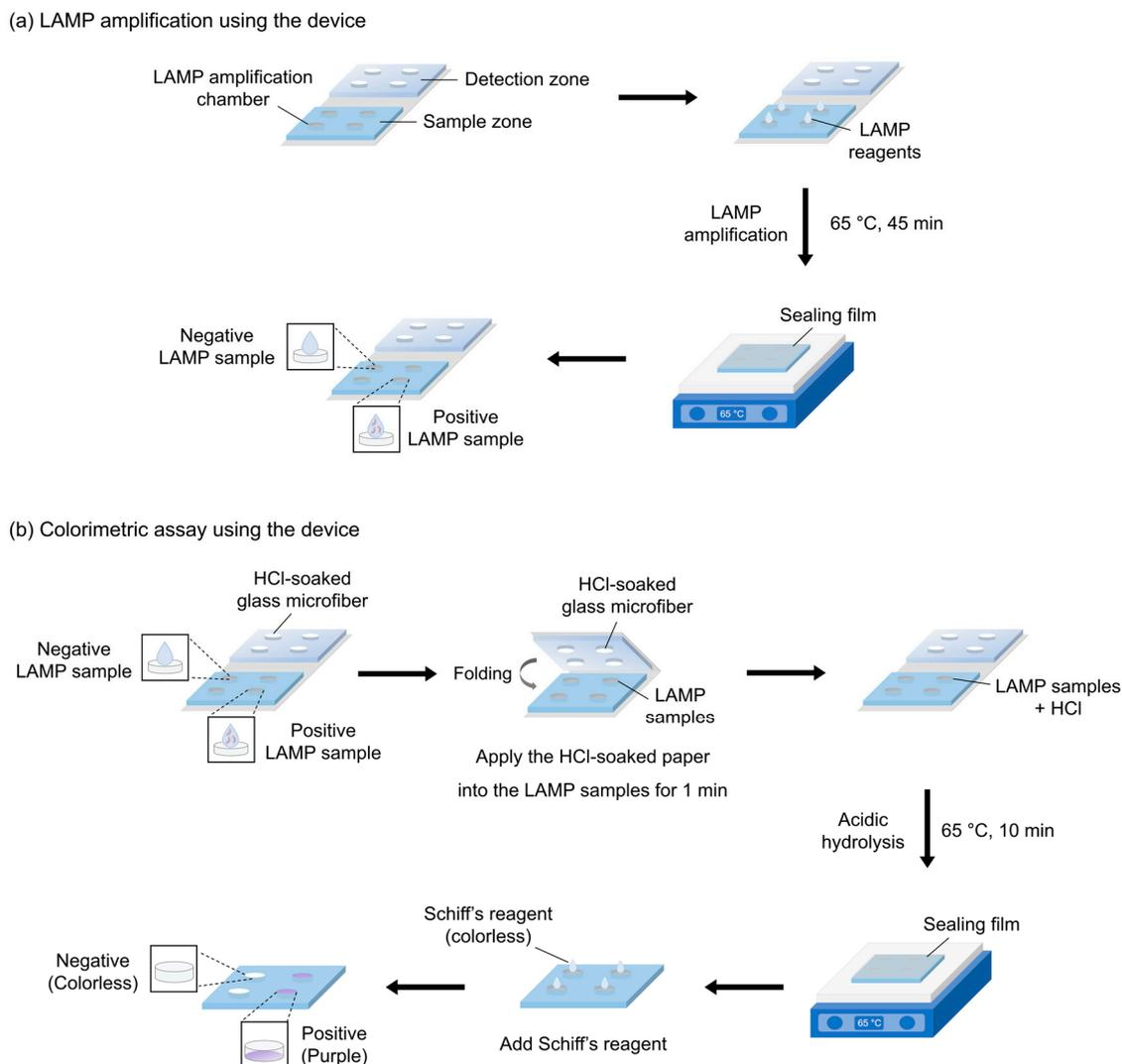
**Figure 2.** Illustration showing the overall operation process of the foldable microdevice. (a) Process of LAMP amplification and (b) colorimetric assay using the device.
