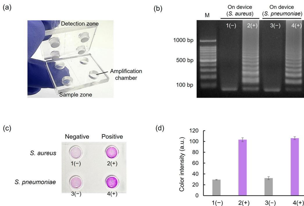
**Figure 9.** LAMP amplification and colorimetric assay performed using the foldable microdevice. (a) Photos showing the structure of the foldable microdevice. (b) Results of the agarose gel electrophoresis of the LAMP amplification performed using the microdevice. (c) Results of the colorimetric assay performed using the microdevice, and (d) analysis results using a color intensity graph.
