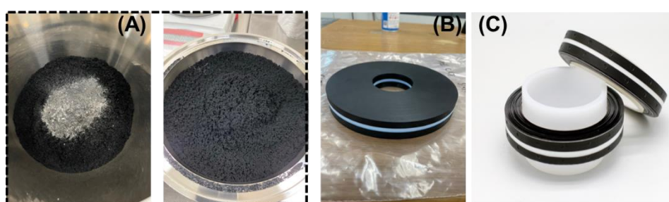
Figure S1: Fabrication of LPEG-PTFE composite and sensor strips.
