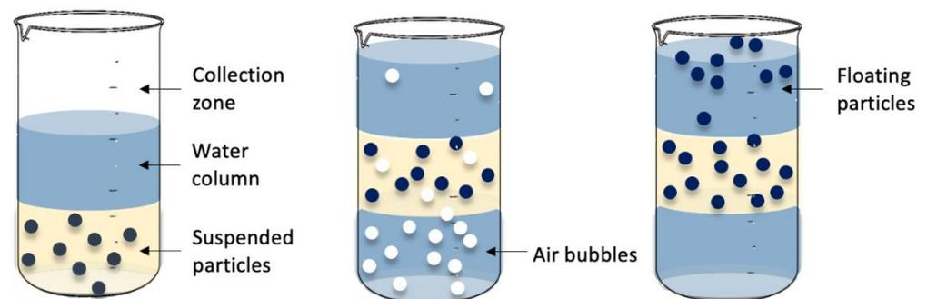
**Figure 4.** Steps of flotation principle.
