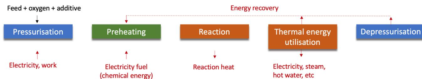
**Figure 5.** Basic diagram for supercritical water oxidation processes.
