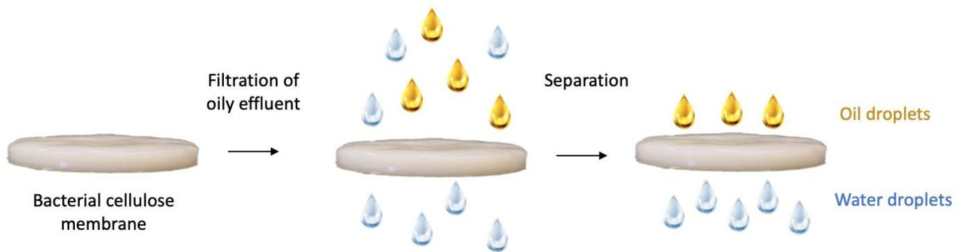
**Figure 7.** Schematic representation of oil-water separation process using BC as filter membrane.
