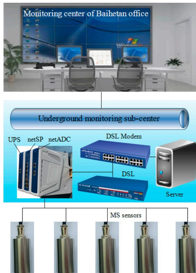
Figure 3. Components and communication mode of the MS system.
