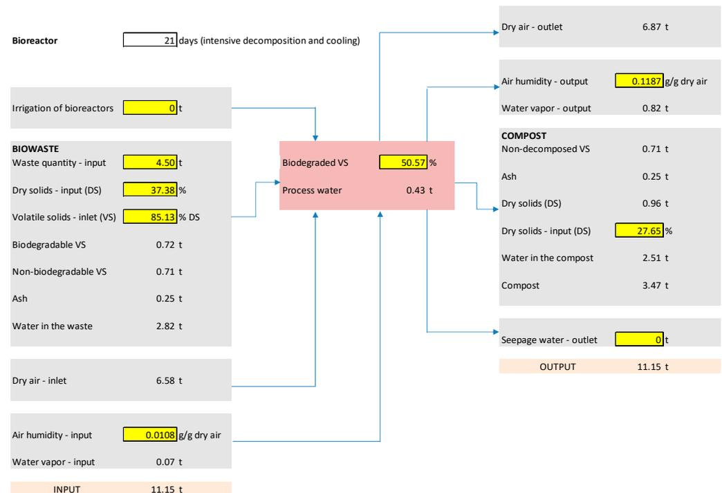
**Figure 2.** Mass balance of the aerobic biodegradation process of a biowaste sample (Excel worksheet screenshot).
