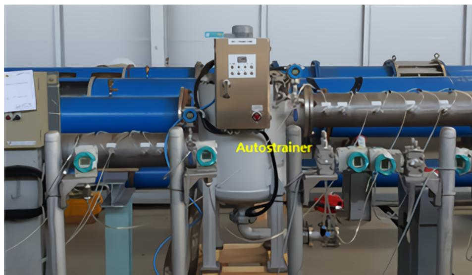
**Figure 10.** Pressure test of the autostrainer.
