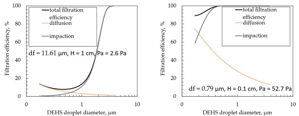
**Figure 9.** Theoretical filtration efficiency and pressure drop (PP fibres left graph, PLA fibres right graph).
