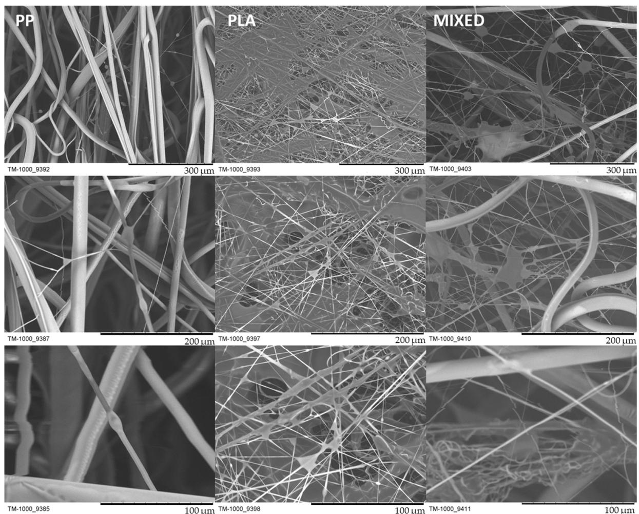
**Figure 11.** The filtration structure after loading study tests with DEHS droplets.
