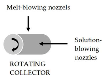
**Figure 3.** Scheme showing of positioning the nozzles to the collector.
