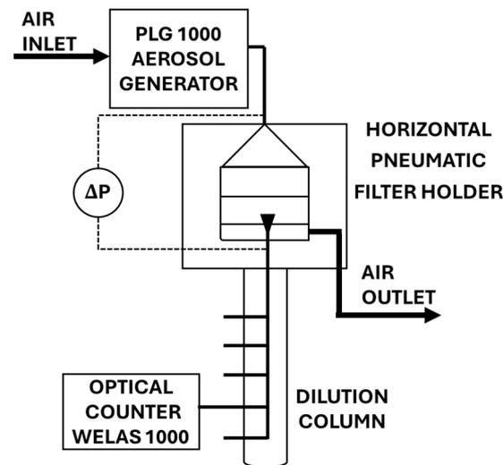
**Figure 4.** Schematic presentation of MFP 1000 HEPA testing rig for filtration droplet with a 0.2–2  $\mu\text{m}$  diameter.
