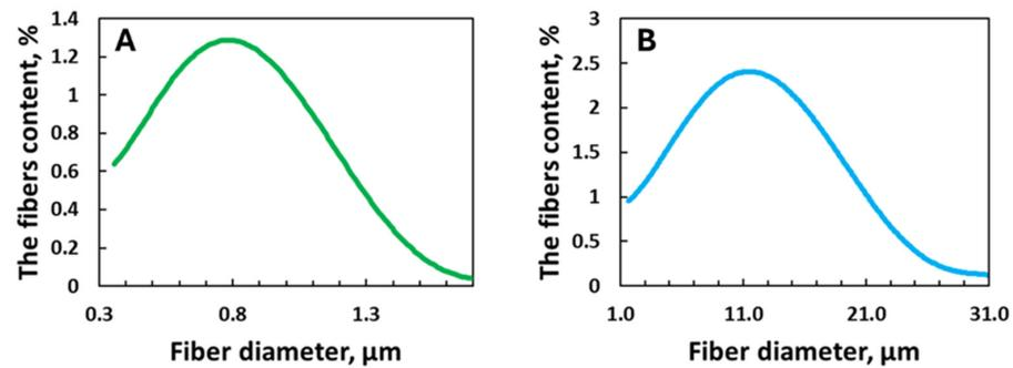
Figure 7. Fibre diameter distribution: (A) PLA fibres, (B) PP fibres.
