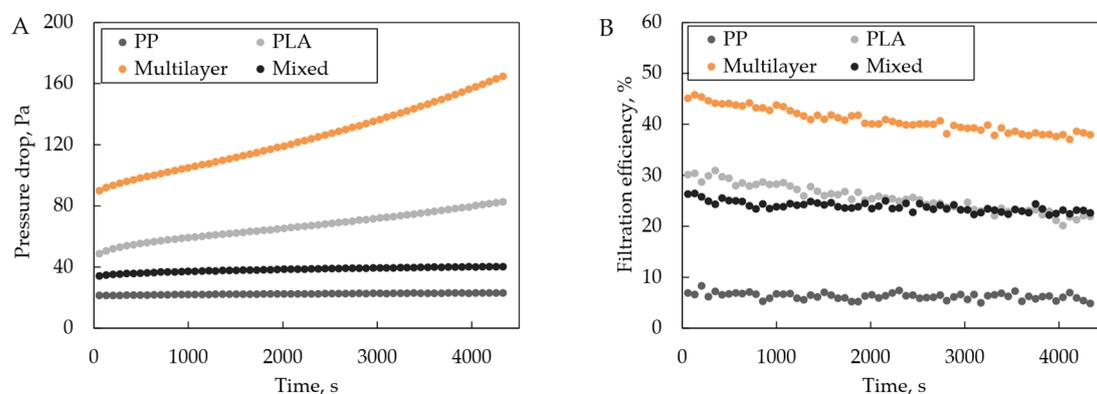
**Figure 10.** The pressure drop (A) and filtration efficiency (B) during the loading study.
