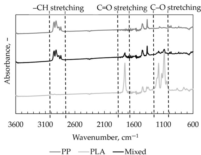
Figure 8. FTIR-ATR spectra of PP fibres, PLA fibres and mixed structure.
