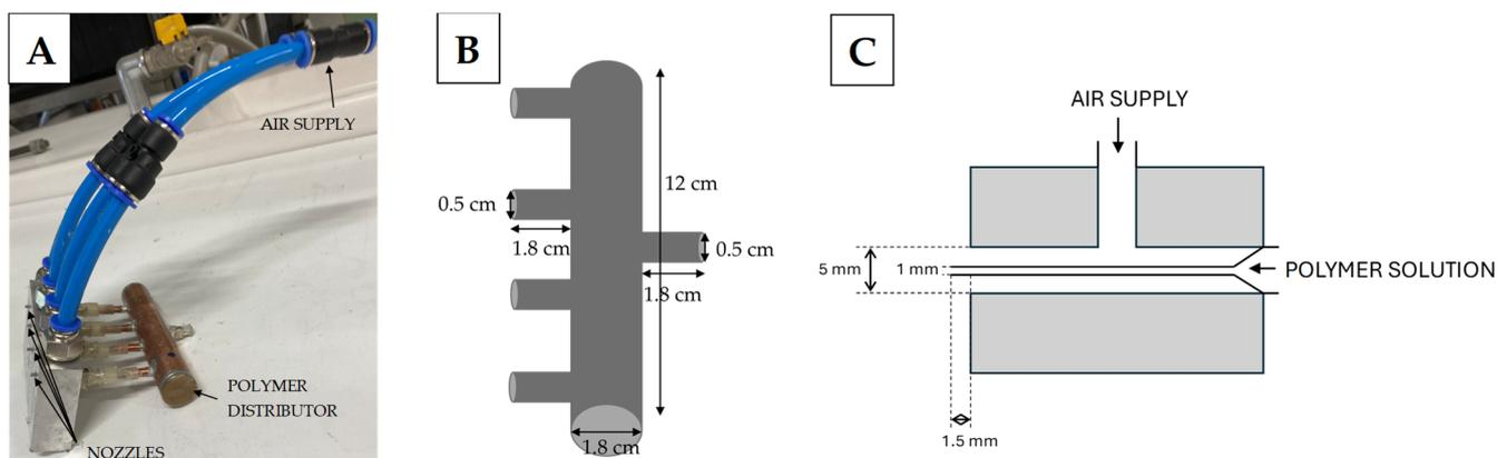
**Figure 1.** The nozzles with the polymer distributor (A), the scheme of the polymer distributor (B), the scheme of nozzle cross-section (C).
