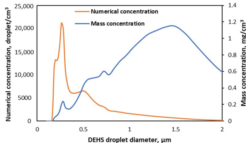
**Figure 5.** The size distributions (0.2–2  $\mu\text{m}$ ) of tested DEHS oil droplets.
