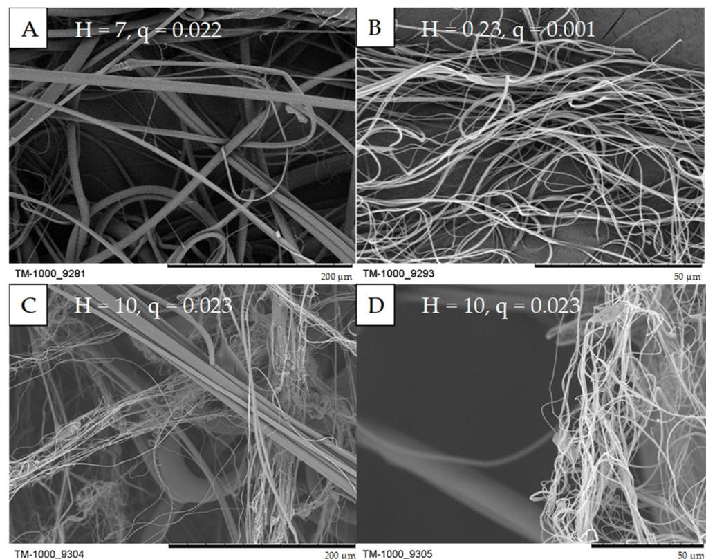
**Figure 6.** SEM photo of obtained filtration structures: (A) PP fibres, (B) PLA fibres, (C) mixed structure, (D) multilayer structure; the thickness of the structures (H, mm) and the surface density ( $q$ , g/cm<sup>2</sup>) were marked in the figure.
