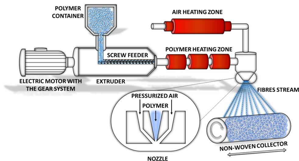
**Figure 2.** The scheme of melt-blowing equipment used to produce non-woven filters. Reproduced with permission [27] Copyright © 2023 Elsevier Ltd. (Amsterdam, The Netherlands).
