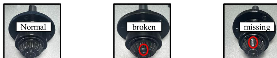
Figure 12. Photographs of the failure gears [29].
