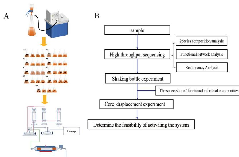
**Figure 5.** (A) Schematic diagram of oligotrophic activation system screening. (B) Rapid screening process in an oligotrophic activation system.
