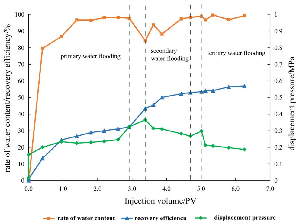
**Figure 3.** Injection pressure, rate of water content, and recovery efficiency were observed with injection volume at various stages of injection.
