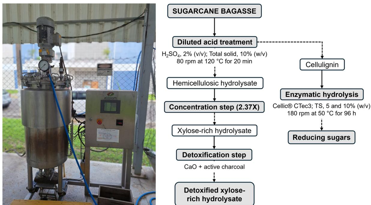
**Figure 1.** General overview of the retrieval of reducing sugars found in the hemicellulosic and enzymatic hydrolysate derived from acid-pretreated sugarcane bagasse, employing a mechanical reactor.
