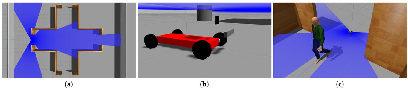
**Figure 5.** Simulation environment: (a) the simulation environment, which is a cross corridor, (b) the car used in the simulation, (c) the pedestrian acting as a dynamic obstacle in the simulation. The blue area in the figure represents the area that the lidar can scan.
