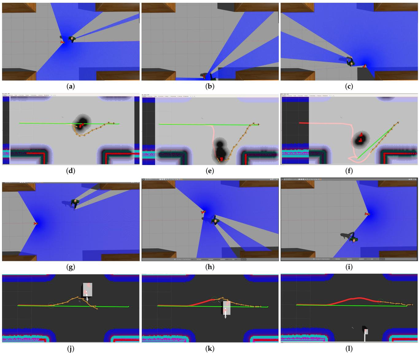
**Figure 8.** (a–c,g–i) Snapshots of the robot using the original TEB and our method to avoid side pedestrians. (d–f,j–l) The rviz screenshots during the operation of the original TEB and our method, respectively, in which the yellow arrows are the TEB poses.
