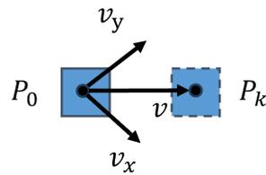
**Figure 3.** Schematic diagram of the obstacle's future position. The solid square area in the figure is the obstacle information detected at the current moment. It has component velocities in the x- and y-directions. The dotted line area is the k-th TEB pose.
