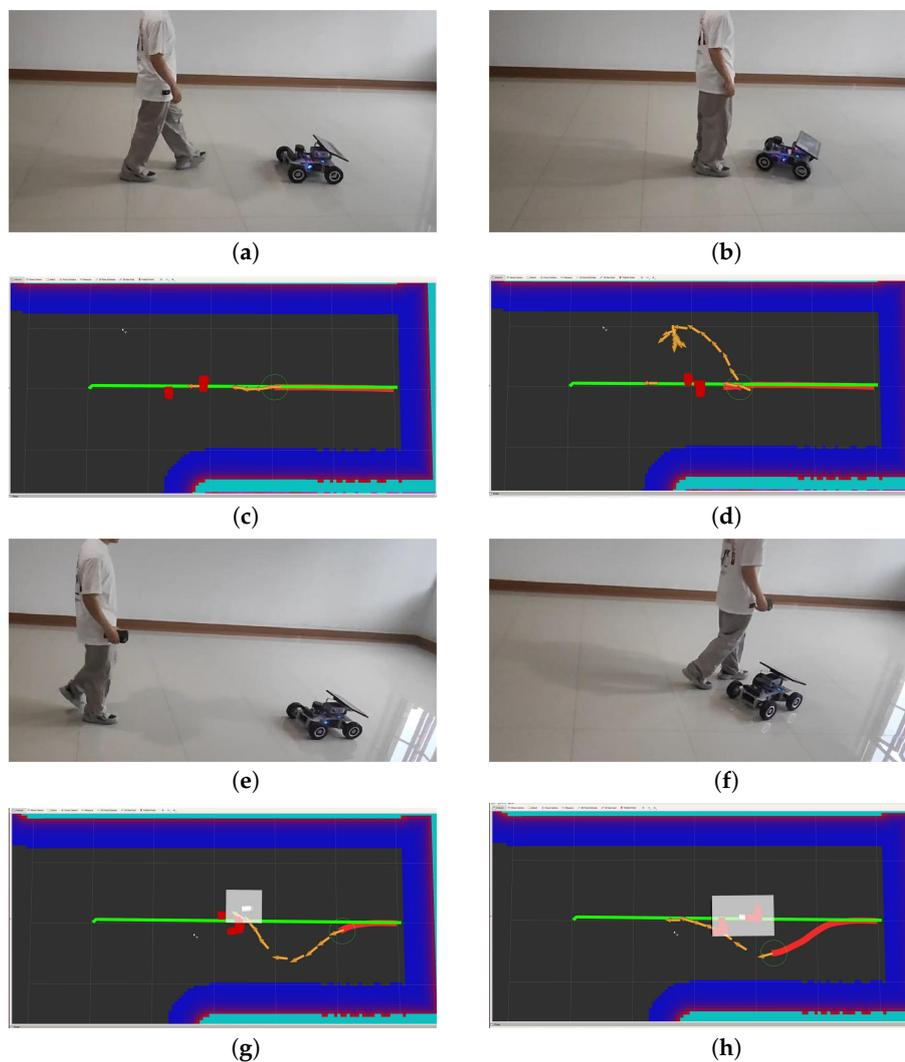
**Figure 12.** Photos of the robot facing oncoming pedestrians and the corresponding rviz screenshots. The yellow arrow indicates the TEB poses, and the red point cloud is the pedestrian scanned by the 2D lidar: (a–d) the original TEB, and (e–h) our method.
