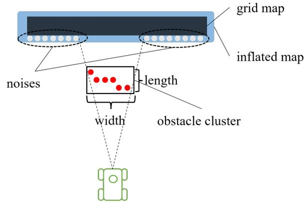
**Figure 1.** Schematic diagram of background point clustering. The points in the figure are the filtered obstacle points: the white points are the noise points, the black rectangle is the obstacle, and the blue area is the inflated obstacle area.
