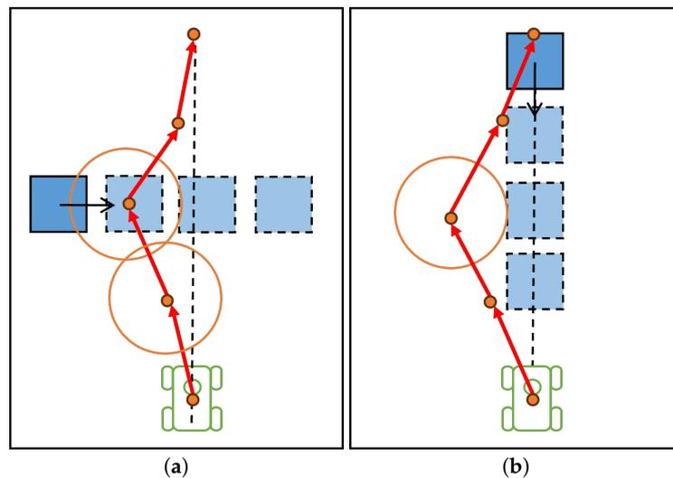
**Figure 4.** Details of improved TEB. This figure presents the details at time  $T_0$ . The local pose sequence of the robot in the figure consists of four red arrows, and the blue square is the obstacle at  $T_0$  while the light-blue squares are the future positions of the obstacle at different times. And the green car represents the robot. The specific calculation process can be referenced in Figure 3 and Equation (16).
