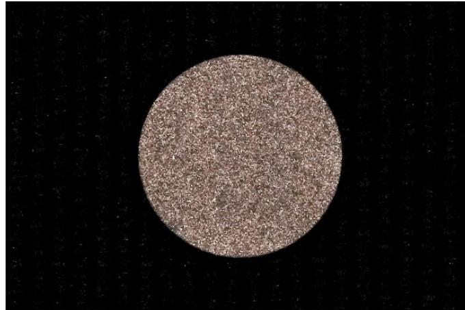
**Figure 1.** Commercially pure Grade 4 moderately roughened titanium disc.
