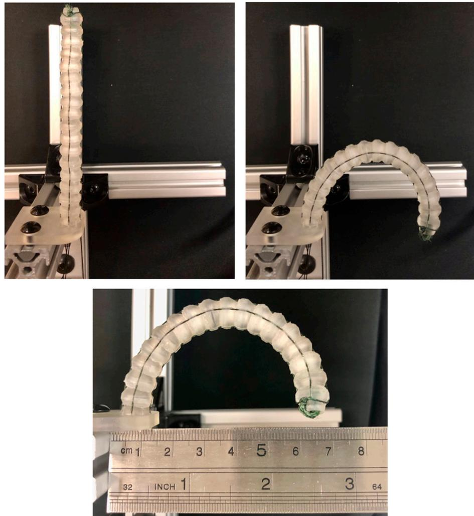
**Figure 18.** Photographs of experimental validations of Model 2 prototype: (**top left**) in undeflected state; (**top right**) in maximum deflection state; (**bottom**) with ruler showing a radius of curvature of approximately 40 mm.
