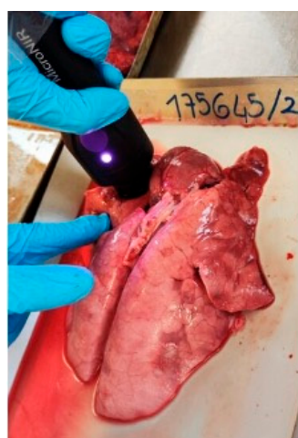
Figure 2. NIR spectra recording of pig lung tissues using the portable spectrometer.
