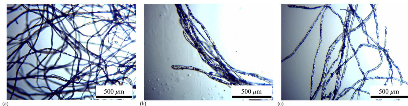
**Figure 3.** Optical microscopy images of magnetizable CMs. (a) Cotton microfibers ( $M_1$ ). (b) Cotton microfibers with honey (light blue) and silver microparticles (gray spots on cotton microfibers) ( $M_3$ ). (c) Cotton microfibers with honey (light blue), silver microparticles (gray spots on cotton microfibers), and CI (dark spots) ( $M_4$ ). See the main text and Table 2 for details.
