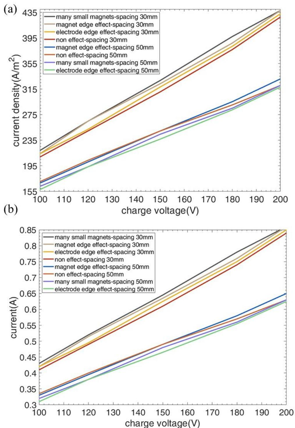
**Figure 10.** (a) Current density vs. charging voltage and (b) current vs. charging voltage for the various experimental layouts.
