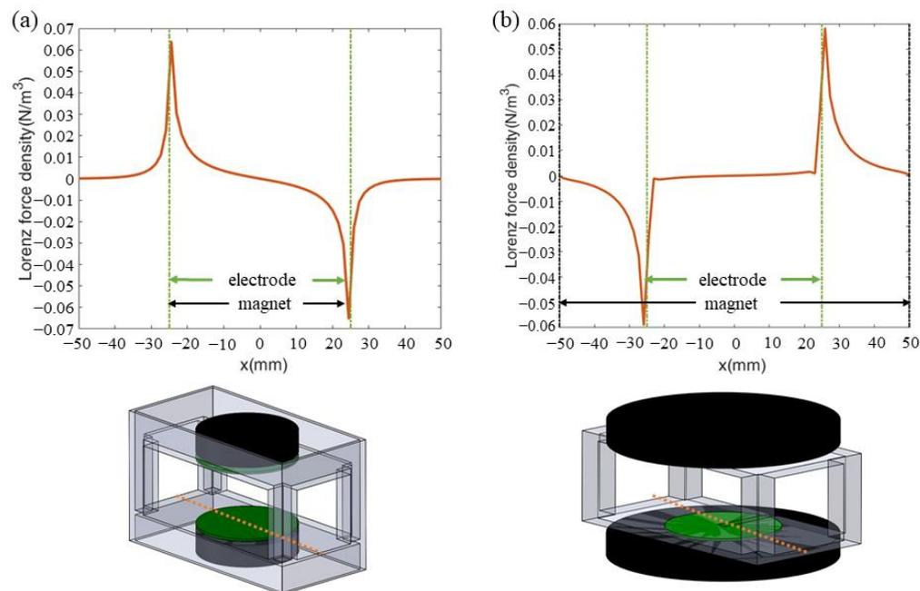
**Figure 9.** The magnitude of the Lorentz force density for electrodes with a distance of 30 mm. The orange dashed line represents the central axis on the electrode plate surface. (a) The Lorentz force density generated by the magnet edge effect at the electrode's edge exhibits a maximum value of approximately  $0.065 \text{ N/m}^3$ . (b) The Lorentz force density generated by the electrode edge effect at the electrode's edge exhibits a maximum value of approximately  $0.058 \text{ N/m}^3$ .
