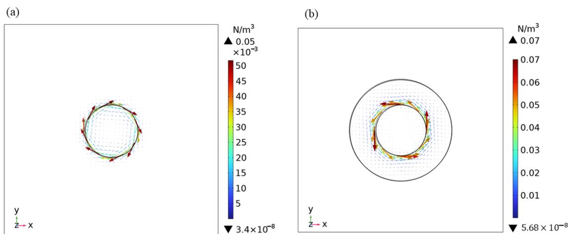
**Figure 7.** Simulation of the Lorentz force density on the lower electrode plate surface of the experimental configuration depicted in Figure 3. (a) When both the magnet and electrode plate have a diameter of 50 mm, the resulting Lorentz force is clockwise. (b) With a magnet diameter of 100 mm and an electrode plate diameter of 50 mm, the resulting Lorentz force is counterclockwise.
