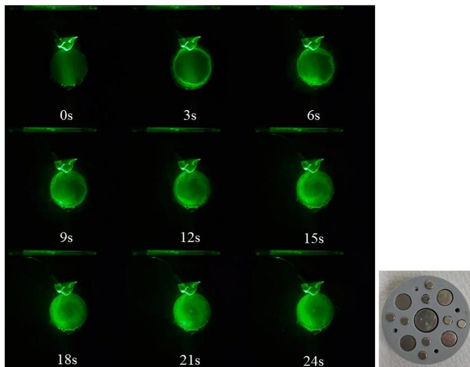
**Figure 11.** Top view of the sequential images of the bubbles' detachment for the electrode influenced by multiple small magnets under the electrode. The extra plot shows the arrangement for the multiple small magnets under the electrode.
