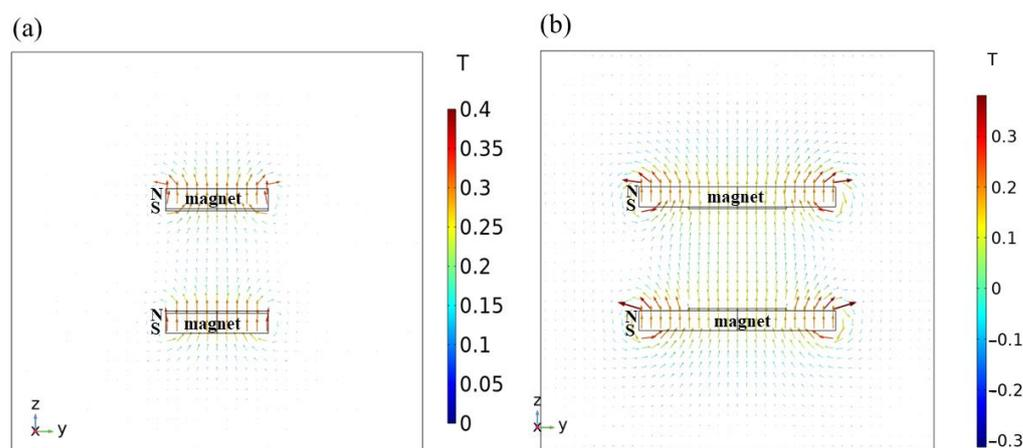
**Figure 4.** Simulation of magnetic flux density. (a) When both the magnet and electrode plate have a diameter of 50 mm, the electrode plate is subjected to the magnet edge effect, with magnetic field lines oriented horizontally at the edge. (b) With a 50 mm diameter electrode plate and a 100 mm diameter magnet, a uniform magnetic field is present on the surface of the electrode plate in a vertical orientation.
