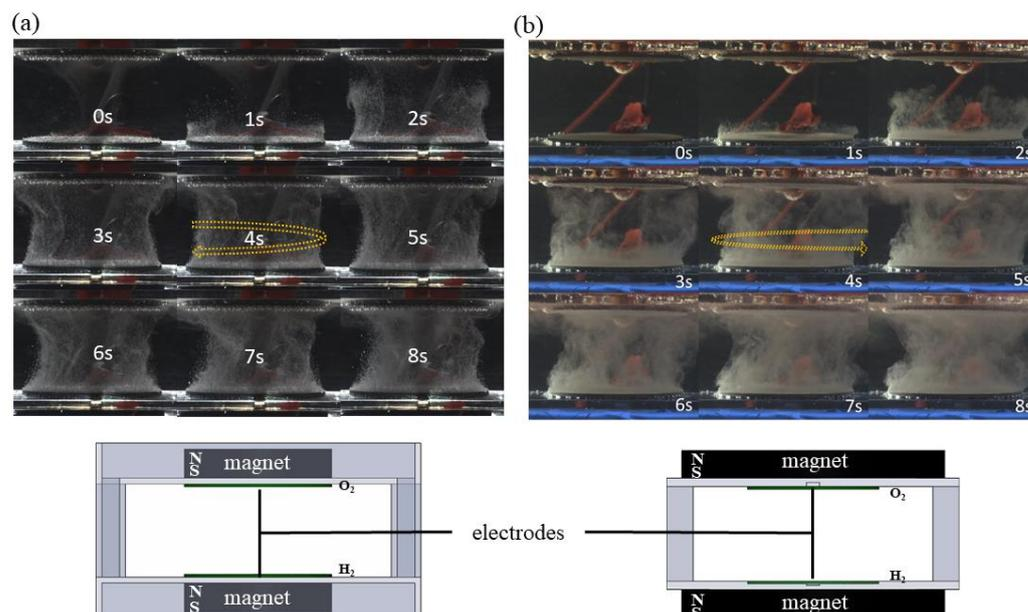
**Figure 6.** Sequential images of hydrogen gas bubbles rotating at the surface of the electrode plates at 100 V voltage and a 30 mm electrode plate spacing. (a) Under the influence of magnet edge, the bubbles rotate clockwise. (b) Under the influence of electrode edge, hydrogen gas bubbles rotate counterclockwise. The arrow indicates the rotating direction of the bubbles.
