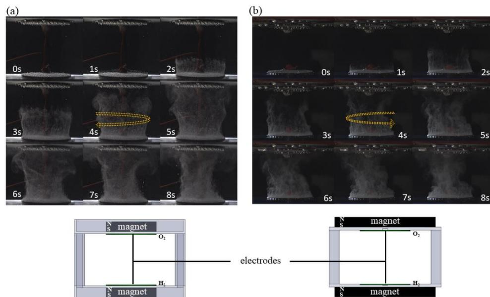
**Figure 3.** Sequential images of hydrogen gas bubbles rotating at the surface of the electrode plates at 100 V voltage and 50 mm electrode plate spacing: (a) under the influence of magnet edge, the bubbles rotate clockwise; (b) under the influence of electrode edge, hydrogen gas bubbles rotate counterclockwise. The arrow indicates the rotating direction of the bubbles.
