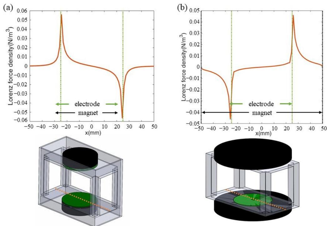
**Figure 8.** The magnitude of the Lorentz force density for electrodes with a distance of 50 mm. The orange dashed line represents the central axis on the electrode plate surface. (a) The Lorentz force density generated by the magnet edge effect at the electrode's edge exhibits a maximum value of approximately  $0.056 \text{ N/m}^3$ . (b) The Lorentz force density generated by the electrode edge effect at the electrode's edge exhibits a maximum value of approximately  $0.045 \text{ N/m}^3$ .
