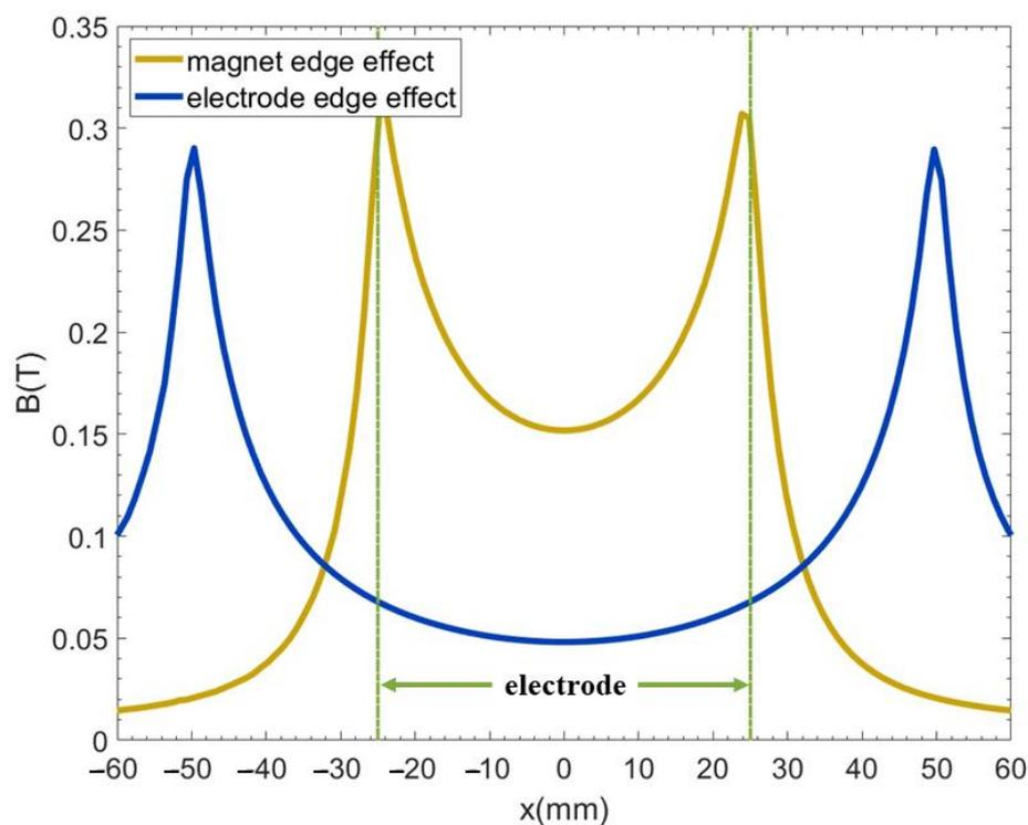
**Figure 12.** The magnetic field intensity distribution on the electrode surface under the influence of magnets with different sizes. The green dashed line represents the electrode plate position. The orange and blue lines denote the range affected by magnets with diameters of 50 mm and 100 mm, respectively.
