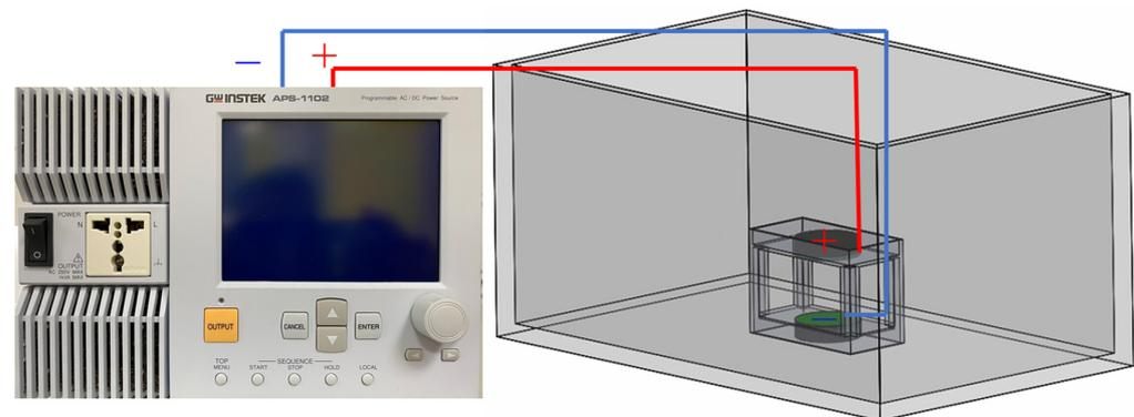
**Figure 2.** The adjustable current is provided by a power supply which connects to the two parallel platinum electrodes. The blue and red line respectively connect the cathode and anode of the electrode plates. The lower and upper electrodes are the cathode and anode which, respectively, generate hydrogen and oxygen.
