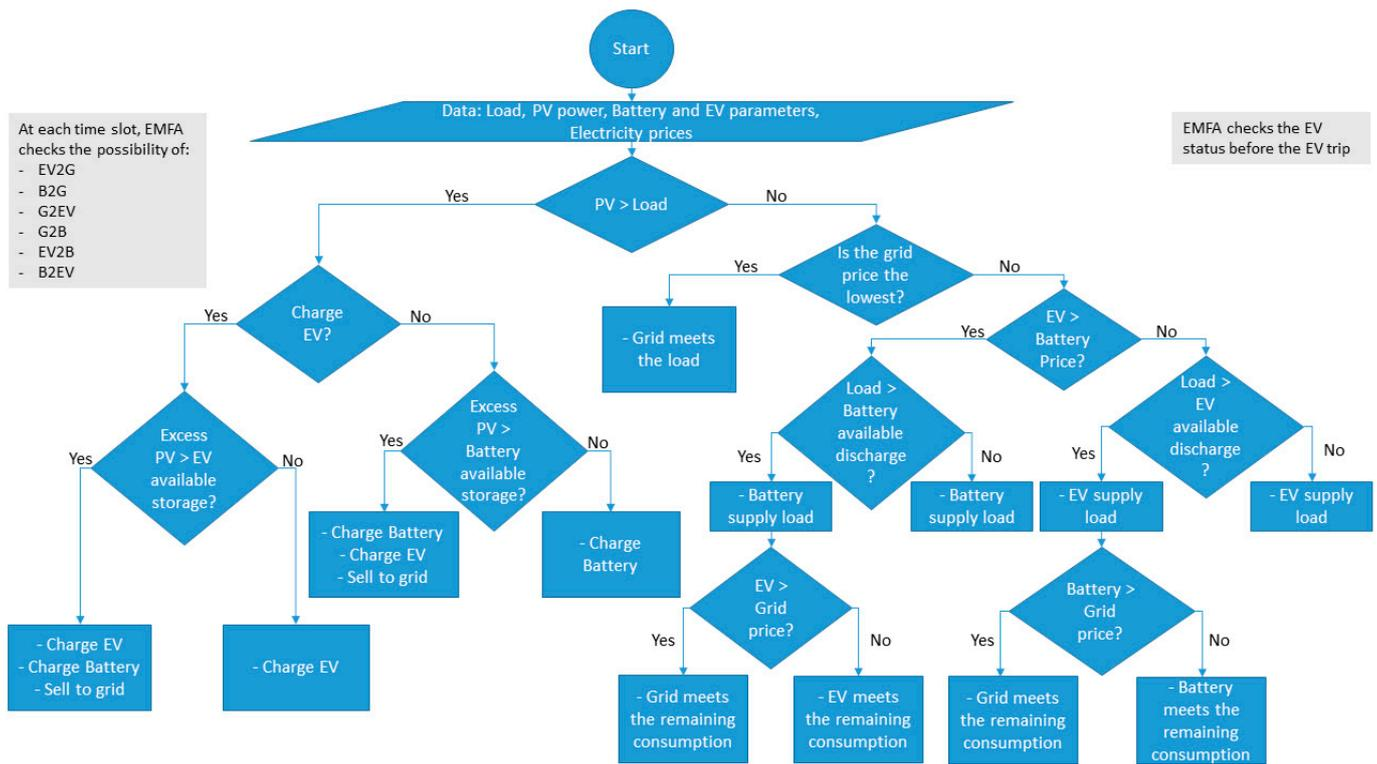
Figure 3. The EFMS algorithm.
