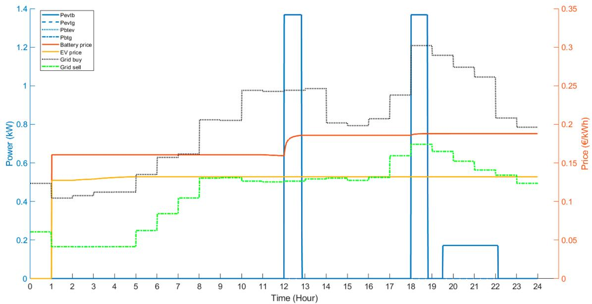
**Figure 11.** Battery and EV battery energy exchange for the third scenario in winter.
