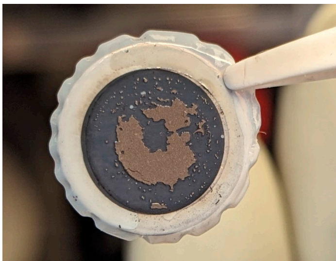
Figure S2. Separator of the cell with unstructured electrodes with plated lithium sticking on it (cathode visible on the backside)
