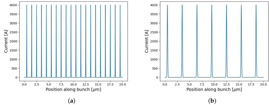
**Figure 2.** (a) 1  $\mu\text{m}$  current profile along the bunch length. The beam is composed of 20 Gaussian functions, each separated by 1  $\mu\text{m}$ . (b) 3  $\mu\text{m}$  current profile along the bunch length, with separation 3  $\mu\text{m}$ .
