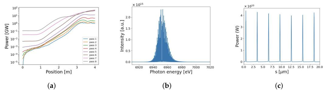
**Figure 8.** Three-dimensional simulation results of UC-XRA FEL with 3  $\mu\text{m}$  modulated electron beams. Each plot shows (a) the gain curve (b) the output spectrum, and (c) the power profile. A maximum power of 44 GW is reached after the sixth pass.
