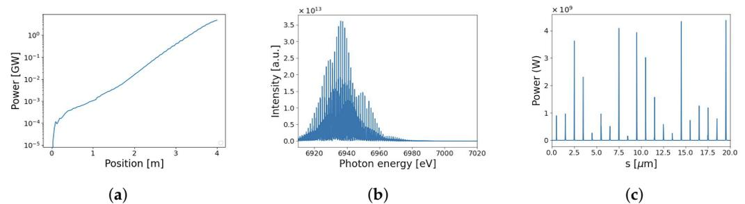
**Figure 6.** Three-dimensional simulation results of a single-pass, non-tapered SASE with 1  $\mu\text{m}$  modulated electron beams. Each plot describes (a) the gain curve, (b) the output spectrum, and (c) the power profile. The maximum output power attainable by single-pass SASE for a 1  $\mu\text{m}$  current profile is 4.5 GW.
