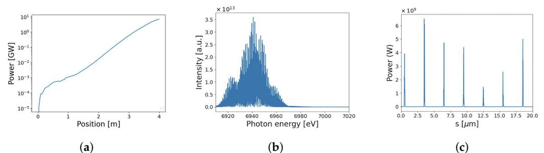
**Figure 9.** Three-dimensional simulation results of a single-pass SASE with 3  $\mu\text{m}$  modulated electron beams. (a) Gain curve, (b) output spectrum, and (c) power profile for SASE with no tapering. The maximum power along the bunch peaks at 6.5 GW.
