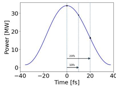
**Figure 7.** Seed profile for the 7th pass of the 1  $\mu\text{m}$  current profile. A 10–20 fs offset of the seed input from the electron bunch length results in a partial decrease of the input seed power.
