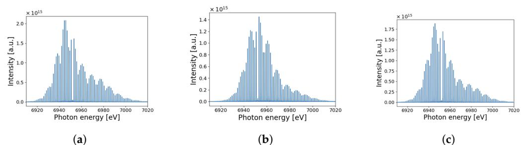
**Figure A1.** Spectra after the seventh round trip of three different UC-XRAFEL runs (a–c) using different random SASE seeds for 1  $\mu\text{m}$  modulated electron beams in order to determine the stability of the UC-XRAFEL seventh pass results using GENESIS 1.3. The spectra are recorded after transmitting through mirror 1.
