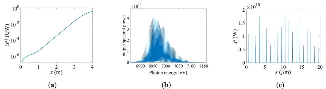
**Figure 4.** 1D SASE simulation results for the 1- $\mu\text{m}$  current modulation. (a) Gain curve, (b) output spectrum, and (c) power profile for single-pass SASE with no tapering. The maximum power peaks at 20 GW.
