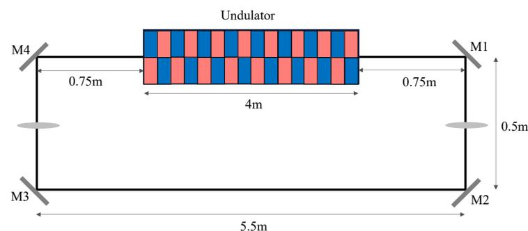
**Figure 1.** The setup of the 12 m round-trip cavity designed for possible use in the UC-XFEL facility.
