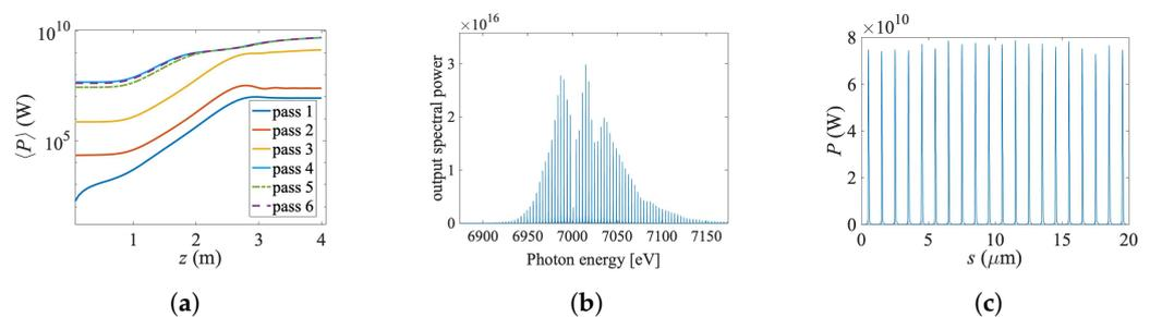
**Figure 3.** 1D UC-XRFEL simulation results for the 1- $\mu\text{m}$  current modulation. (a) The gain curves after each recirculation pass for optimal tapering [37]. (b) The output spectrum after the 5th pass. (c) The power profile of the out-coupled radiation for the 5th pass, with a maximum power along the bunch peaking at 80 GW.
