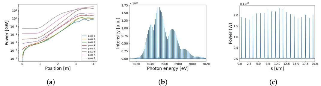
**Figure 5.** Three-dimensional simulation results of UC-XRFEL with 1  $\mu\text{m}$  modulated electron beams. Each plot describes (a) the gain curves after each pass through the cavity, (b) the output spectrum after the 7th pass, and (c) the power profile of the out-coupled radiation for the 7th pass. The maximum output power along the bunch peaks at 25 GW.
