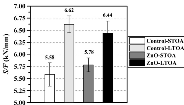
**Figure 8.**  $S/F$  ratio—Control and modified samples under STOA and LTOA condition.
