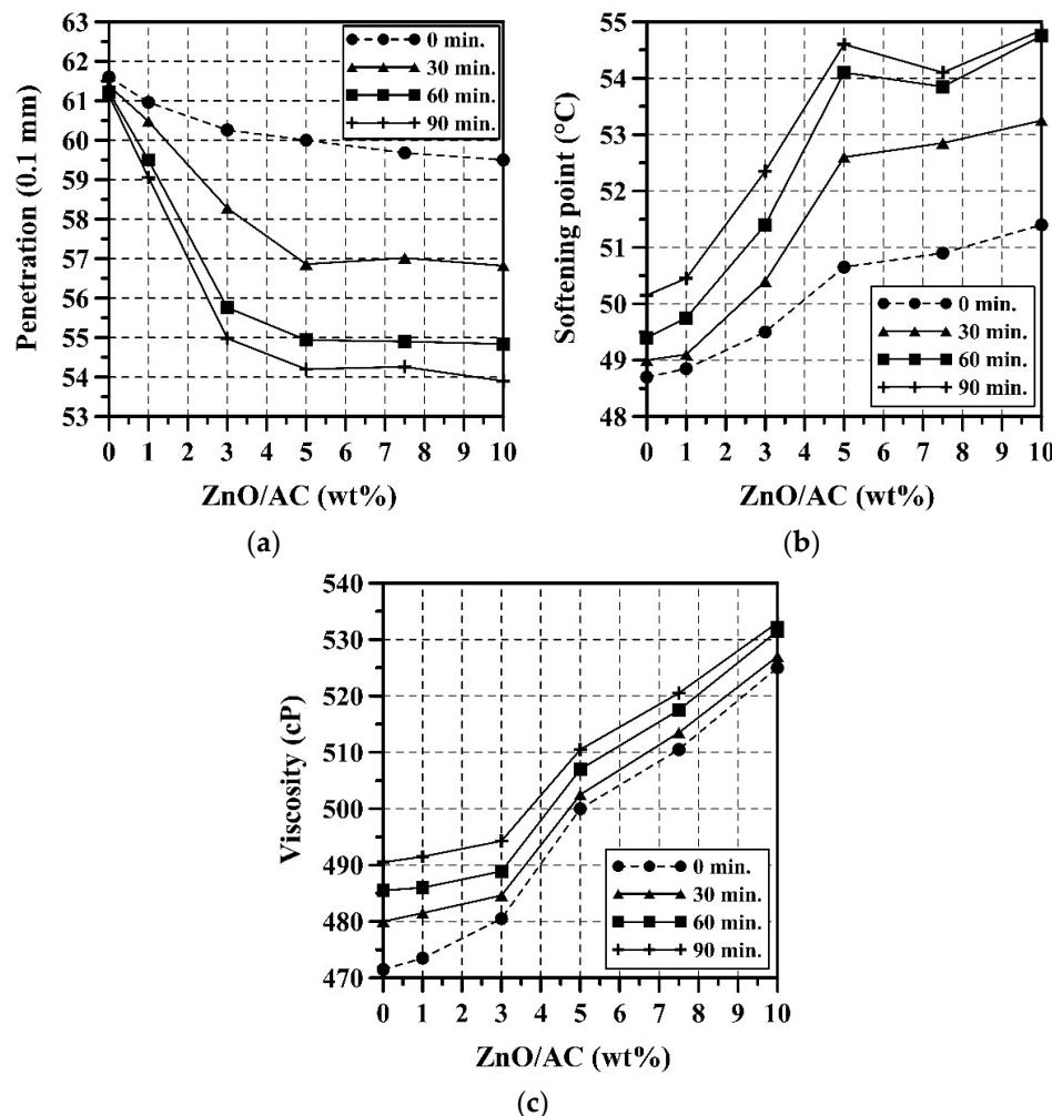
**Figure 3.** Evolution of (a) penetration, (b) softening point, and (c) viscosity with  $\text{ZnO}/\text{AC}$  content and MT.
