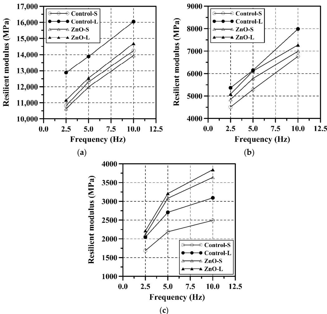
**Figure 10.** RM test results. (a) 10 °C, (b) 20 °C, and (c) 30 °C.
