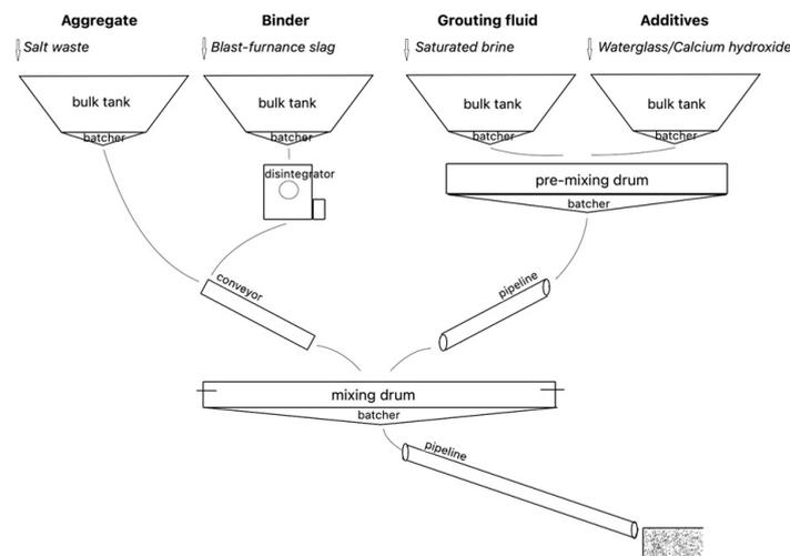
**Figure 7.** Technological scheme of backfill preparation.
