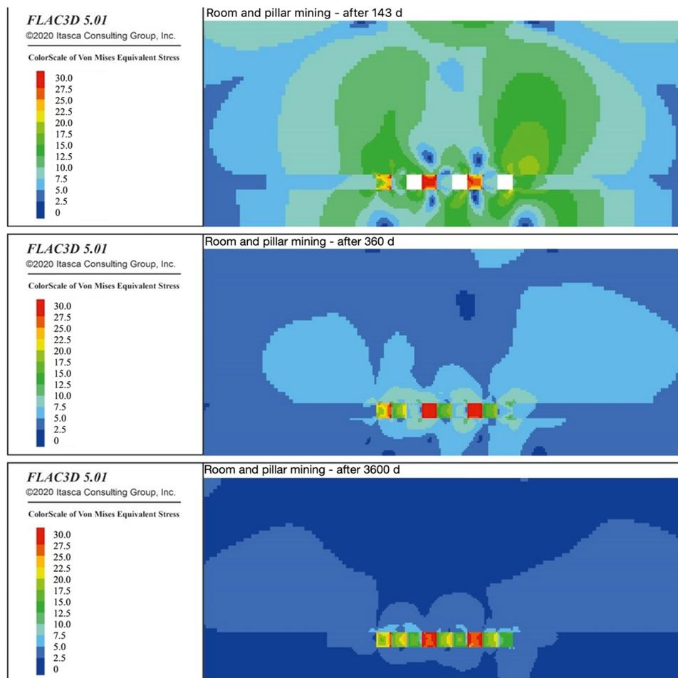
Figure 11. Salt mass behaviour in the mining area, stress distribution.
