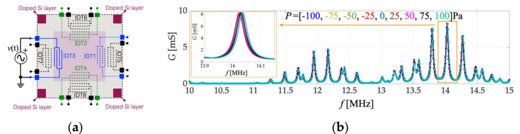
**Figure 2.** Simplified schematic view of the proposed MEMS device configured for the simulation of the electrical admittance (a). Simulated conductance  $G(f)$  of a single IDT as a function of the excitation frequency  $f$  at different pressure  $P$  (b). Enlarged view of a single peak of  $G(f)$  (inset).
