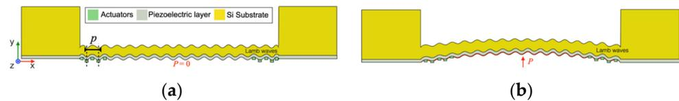
**Figure 1.** Cross-section views of the proposed piezoelectric MEMS pressure sensor without (a) and with (b) the pressure  $P$  applied.
