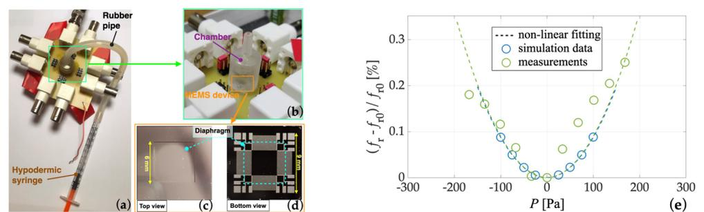
**Figure 3.** Experimental setup employed to test the MEMS pressure sensor (a). Enlarged view of the sealed chamber (b). Top (c) and bottom (d) views of the fabricated MEMS device. Comparison (e) of the simulated (blue circles) and measured (green circles) relative resonant frequency variation and non-linear fittings (dotted curves) as a function of the applied pressure  $P$ .
